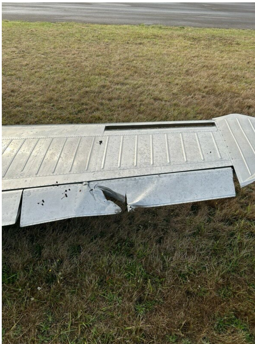
Photograph 3 - Right Aileron (Courtesy of FAA)
