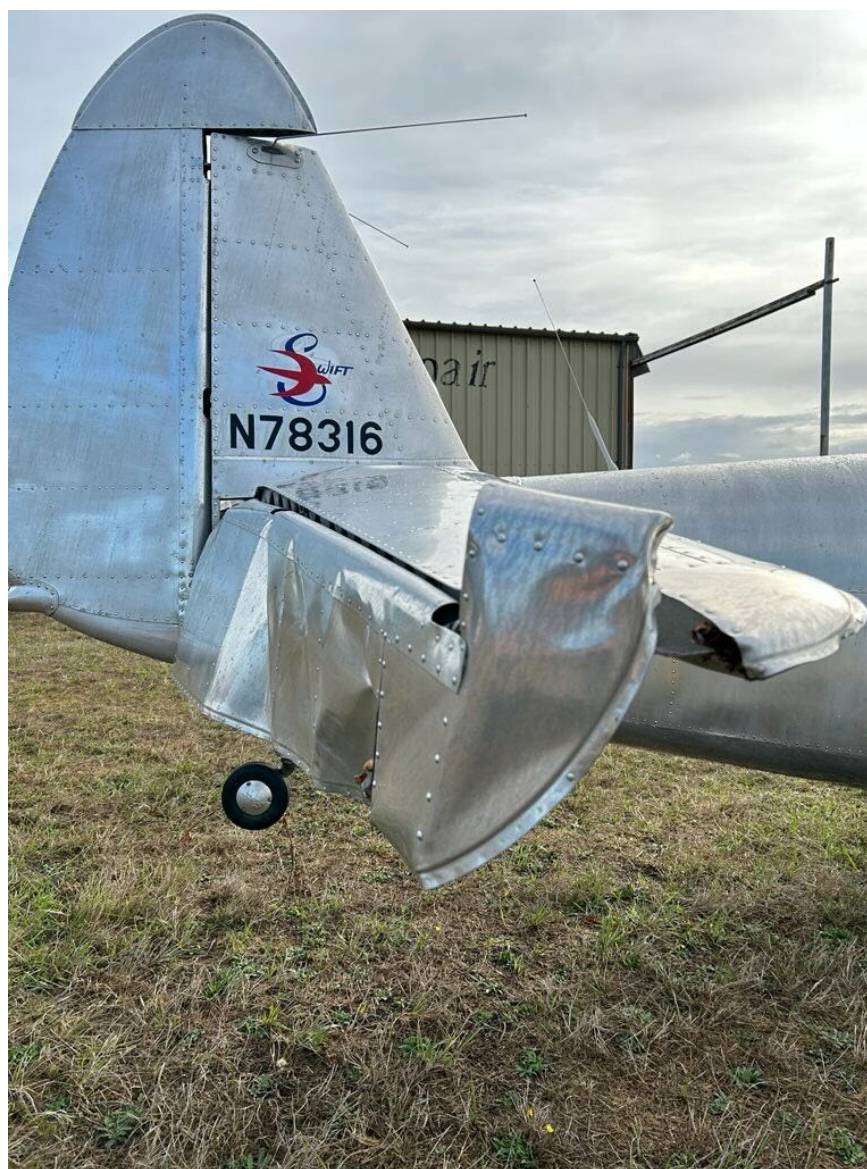
Photograph 4 - Empennage (Courtesy of FAA)
