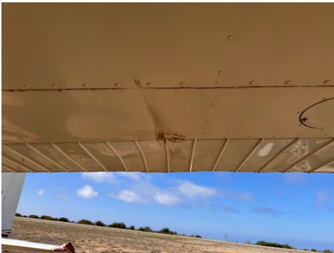
Photograph 2 - Substantial damage to the left aileron. (Courtesy of airport manager)
