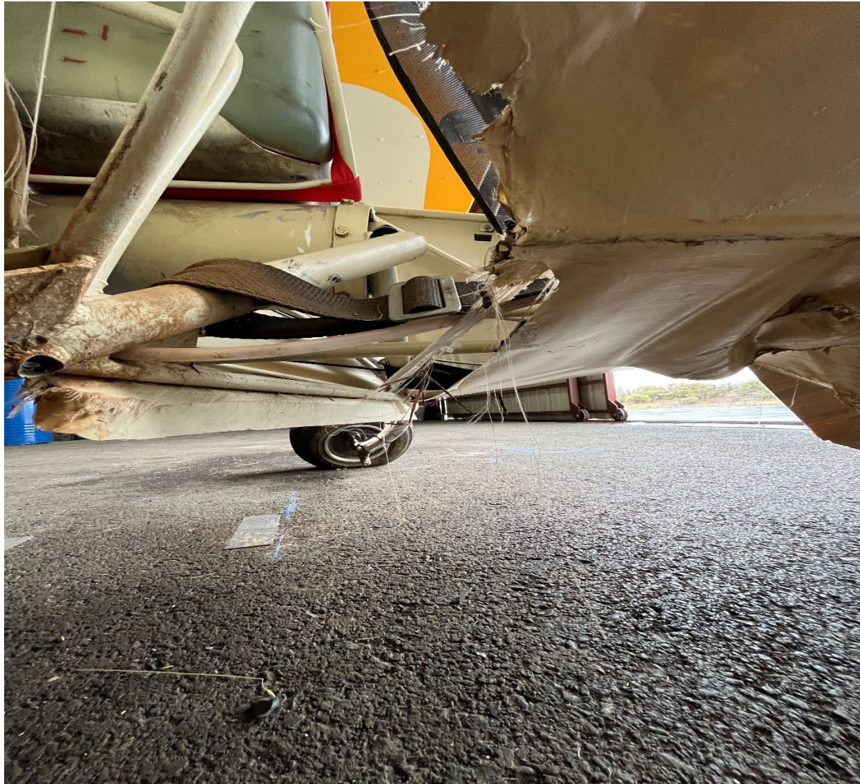
Photograph 2 - View of damage to the bottom fuselage (Courtesy of FAA)
