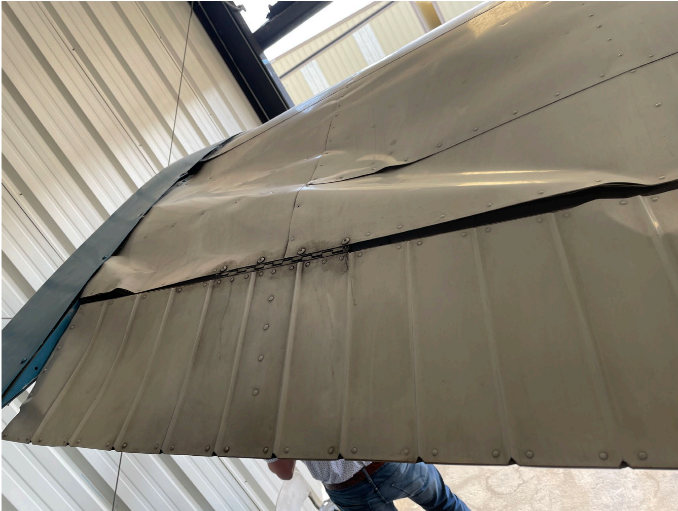
Photograph 2 - A view of substantial damage to the left wing. (Courtesy of the FAA.)
