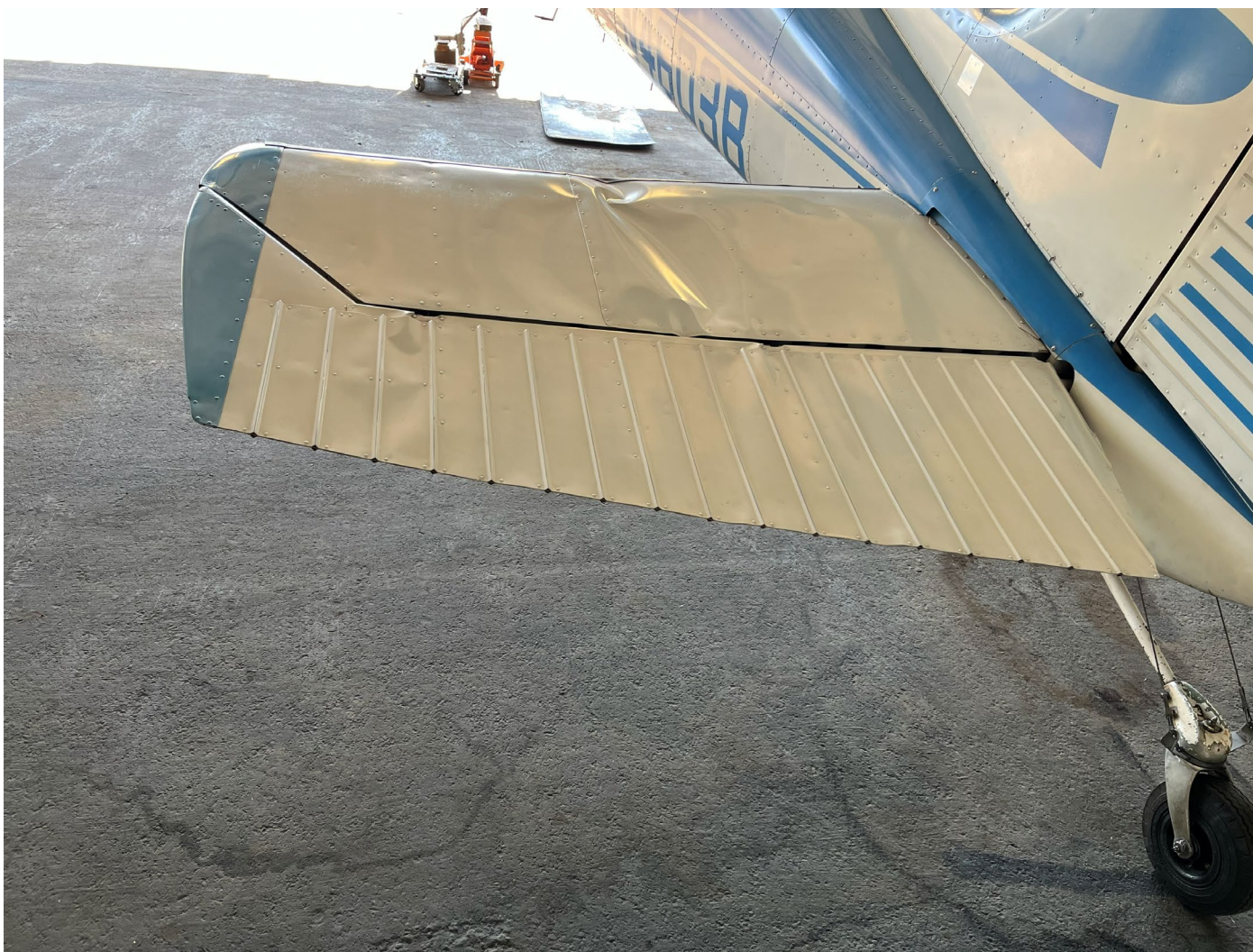
Photograph 3 - A view of the substantial damage to the left horizontal stabilizer. (Courtesy of the FAA.)
