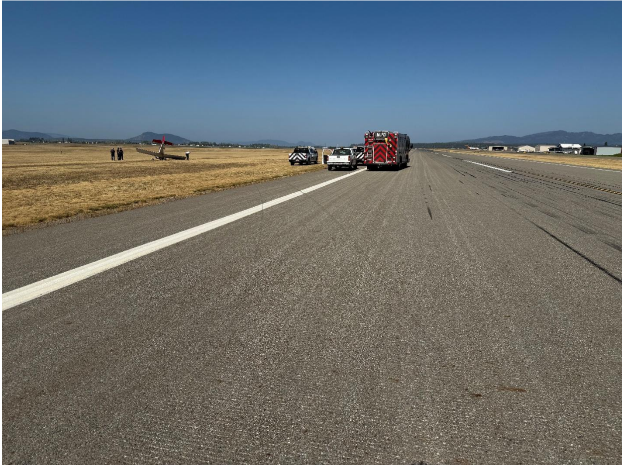
Figure 3: Airplane tire marks, edge of runway, and final location
