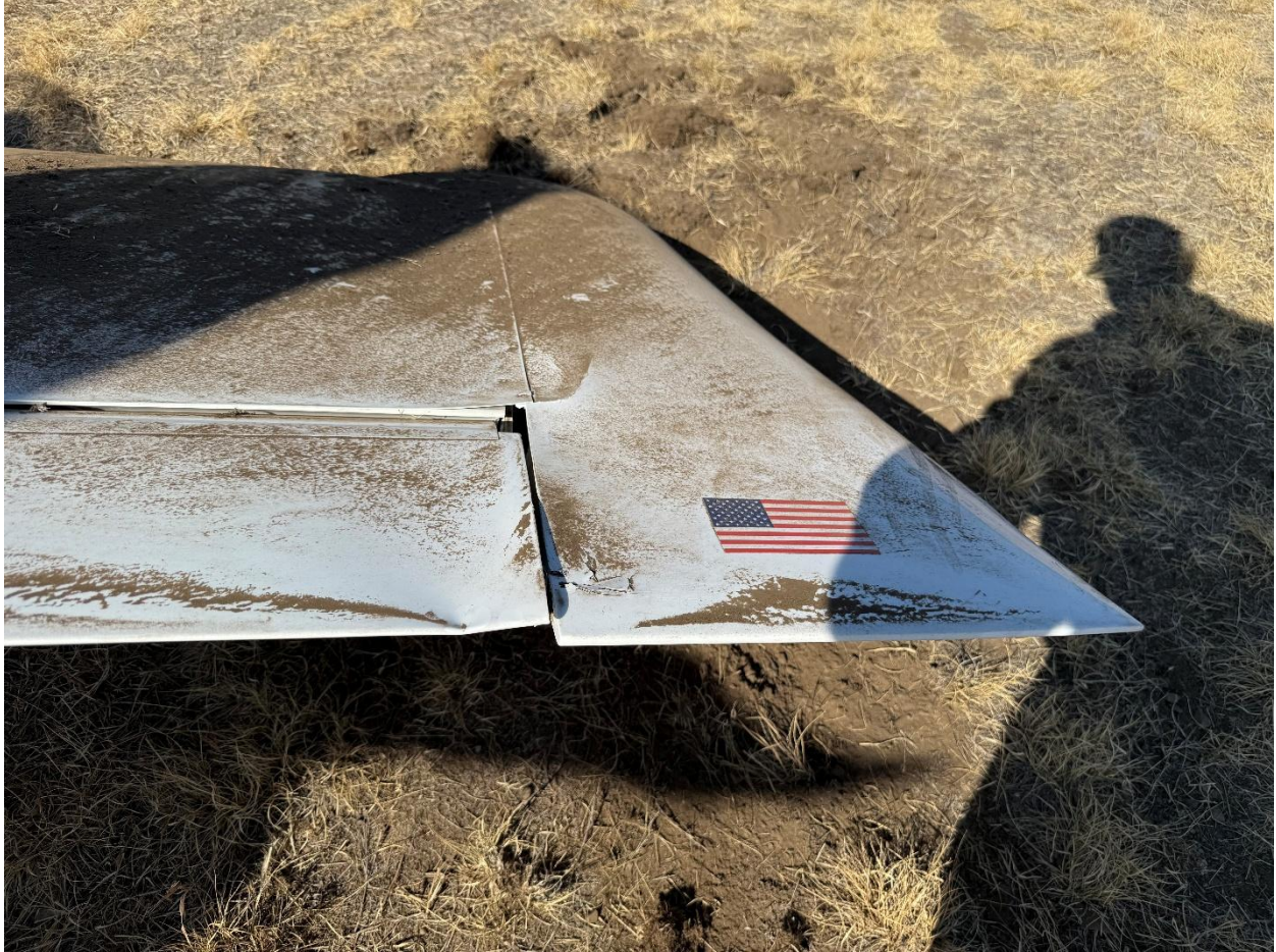
Figure 7: Left wing/aileron damage
