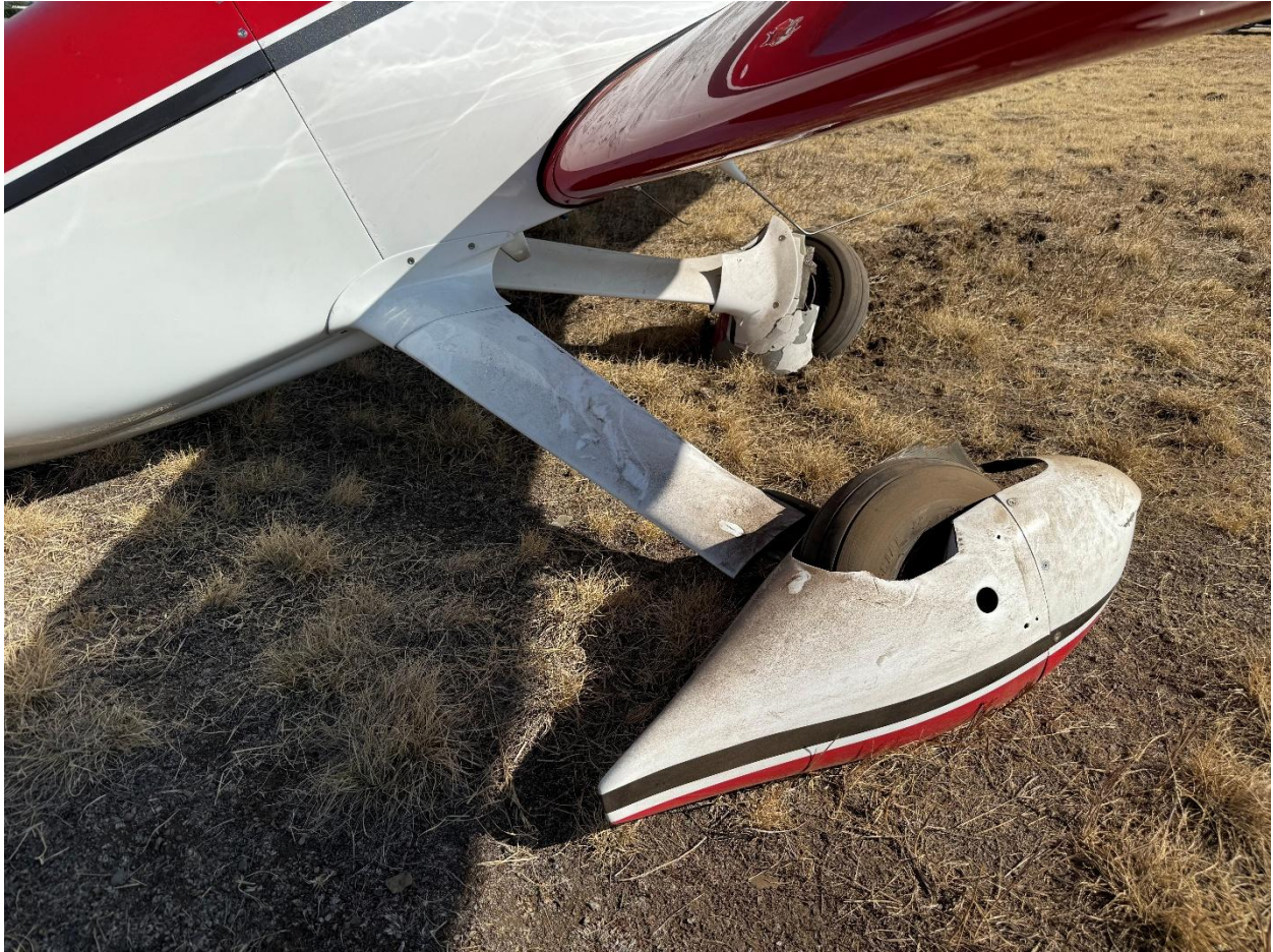
Figure 5: Airplane landing gear damage (left side)
