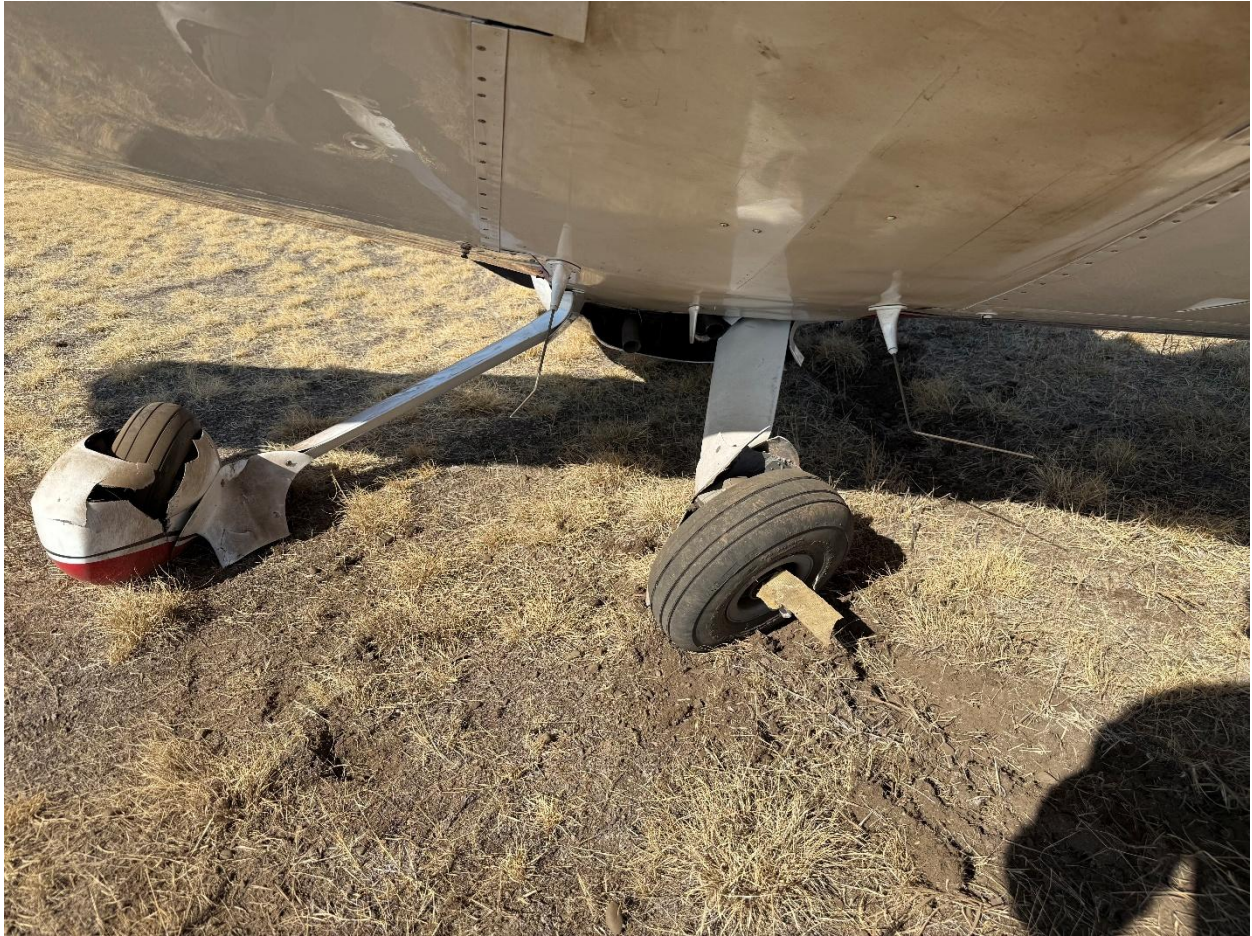
Figure 6: Airplane landing gear damage (from rear)
