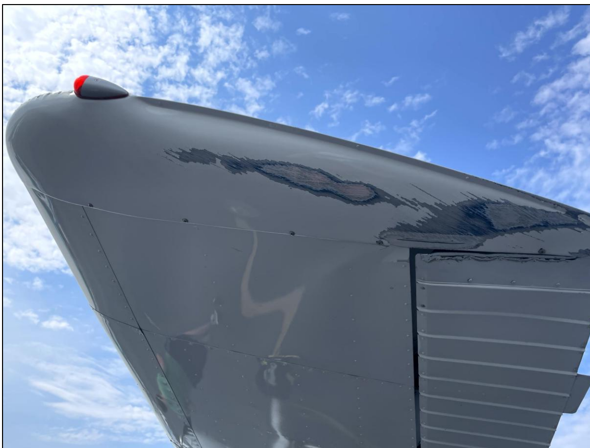
Photograph 2 -Left wing tip fairing and aileron damage. (Courtesy of the pilot)
