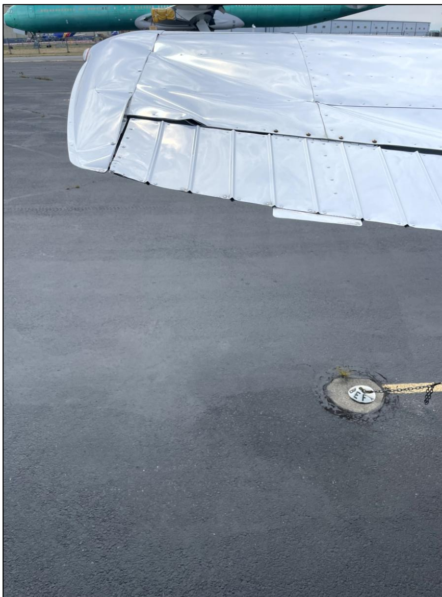
Photograph 1 -Left horizontal stab and elevator damage. (Courtesy of the pilot.)
