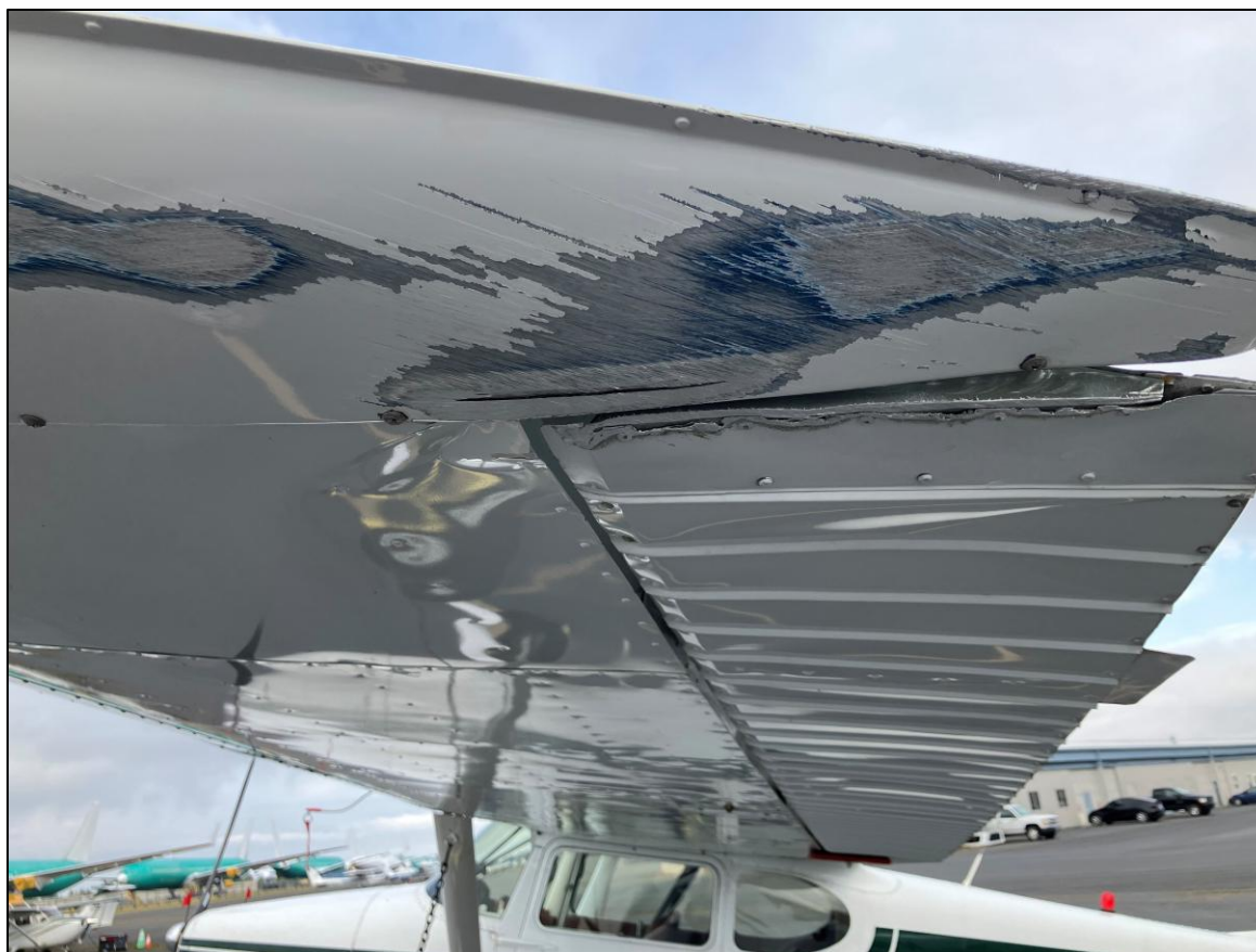
Photograph 3 - Left wing tip fairing damage. (Courtesy of the FAA)
