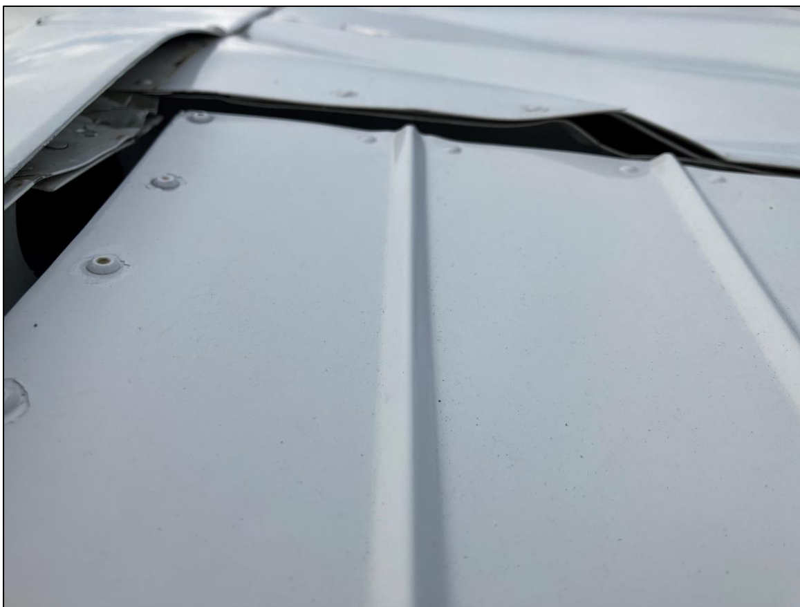
Photograph 4 - Left outboard wing upper surface damage. (Courtesy of the FAA)
