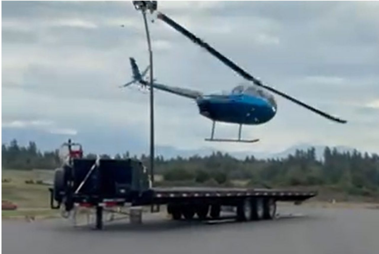
Photo 1 - View of the helicopter's right side tailboom striking light pole (Courtesy of BVS Airport Operations)
