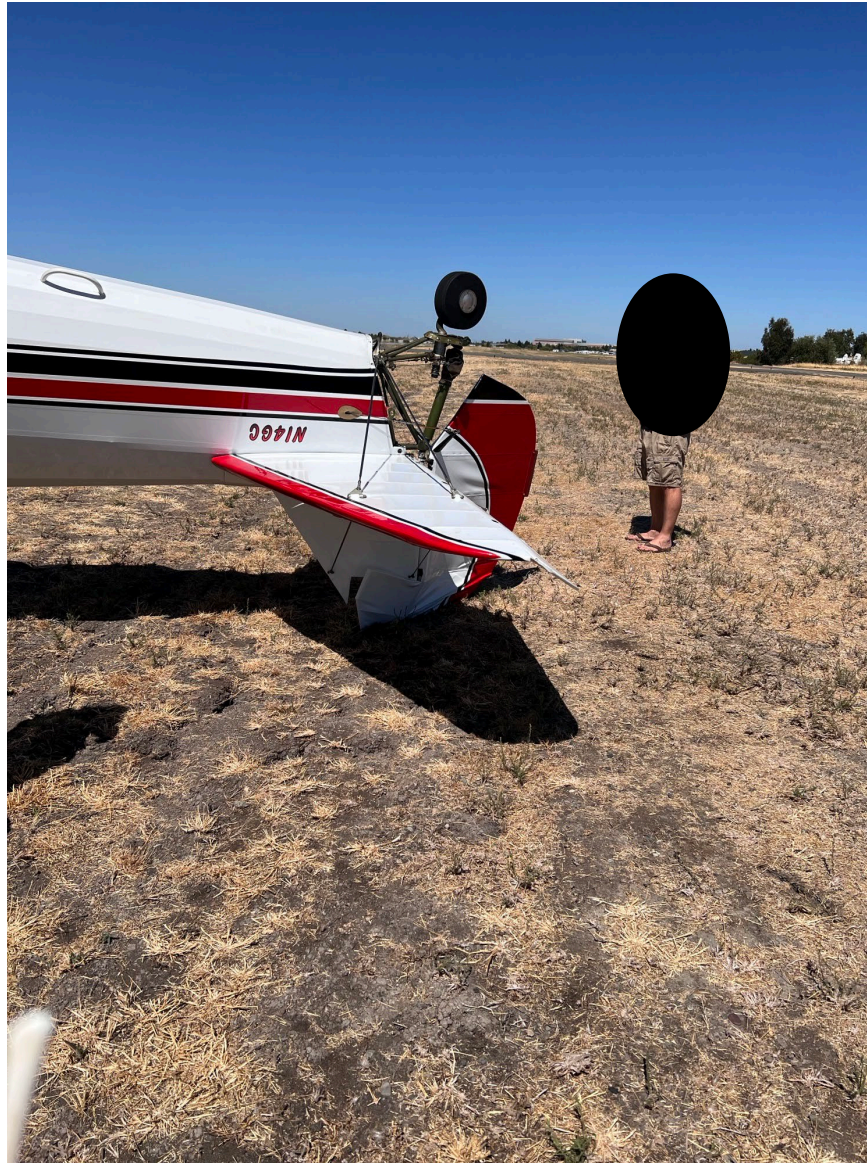
Photograph 2 - View of rudder damage (Courtesy of airport operations)
