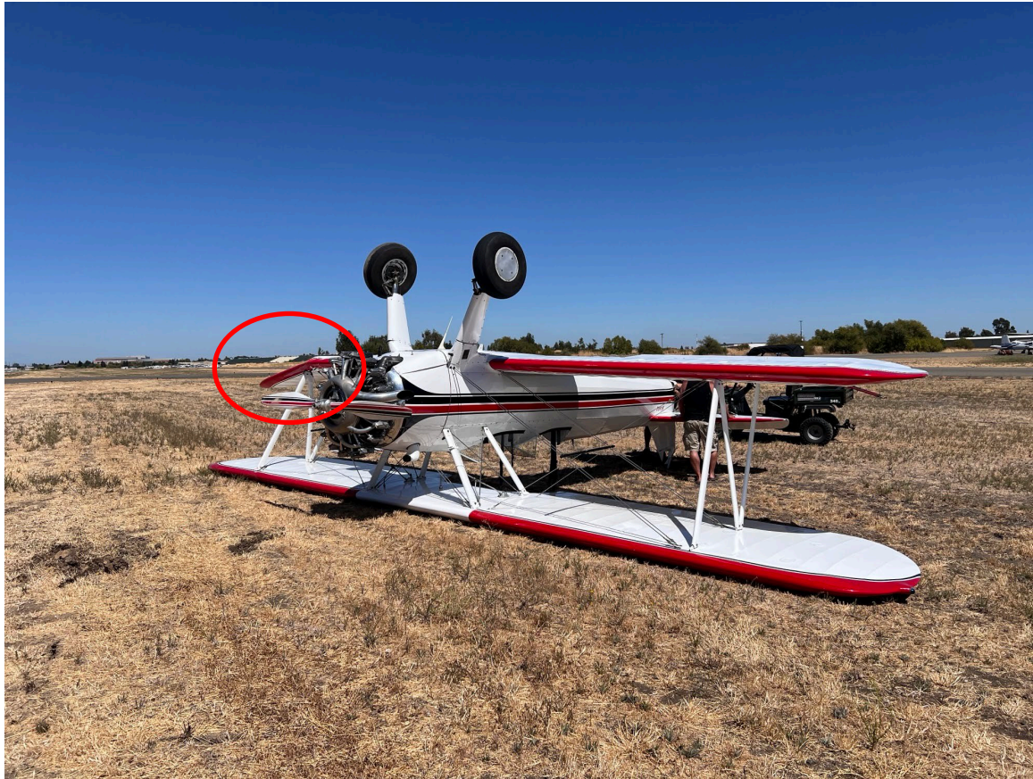
Photograph 1 - View of lower left wing damage (Courtesy of airport operations)
