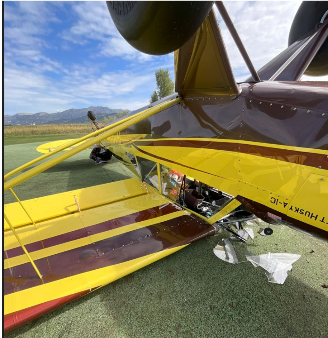
Photograph 1 - Inverted Airplane showing fuselage and tail damage. (Courtesy of Airport Manager)
