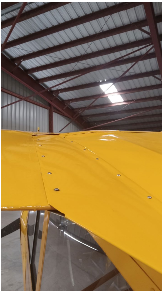
Photograph 2 - Wrinkled Top Wing Skin (Courtesy of Pilot)
