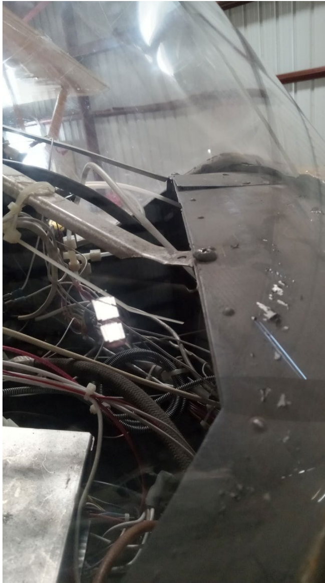
Photograph 4 - Distorted Glare Shield and Support (Courtesy of Pilot)
