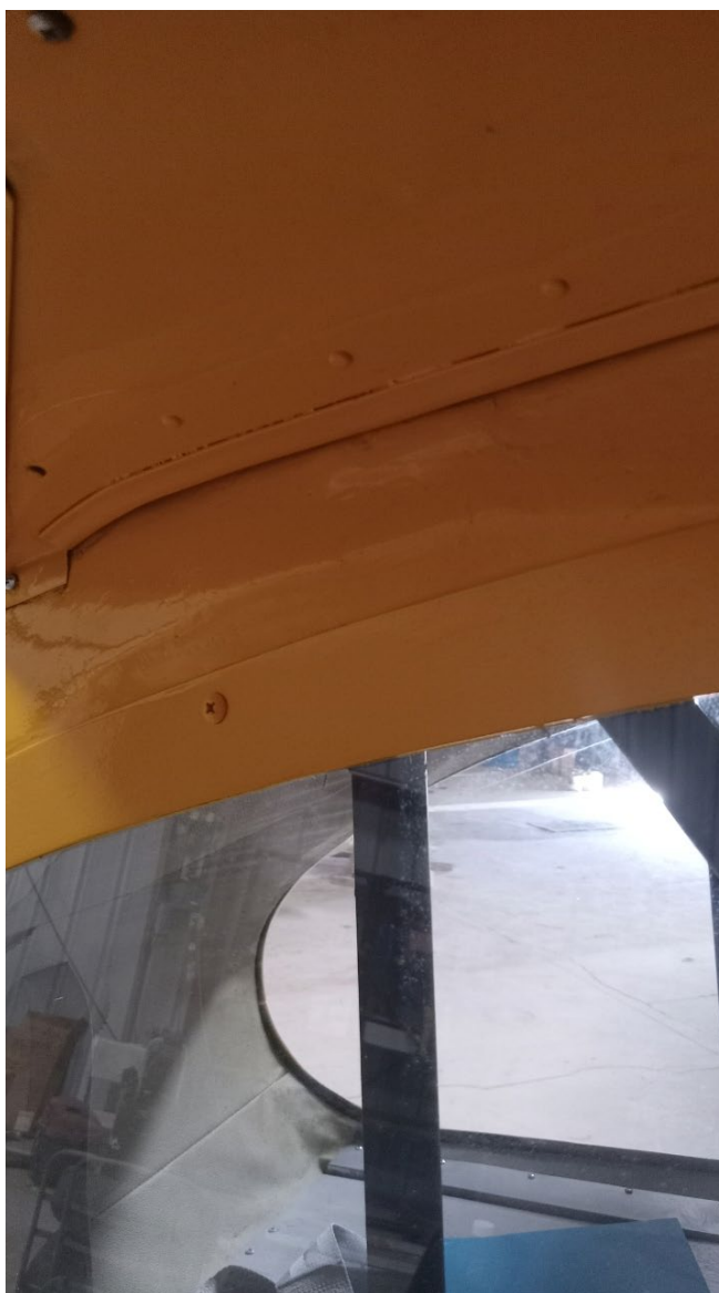
Photograph 3 - Distorted Fuselage Skin (Courtesy of Pilot)
