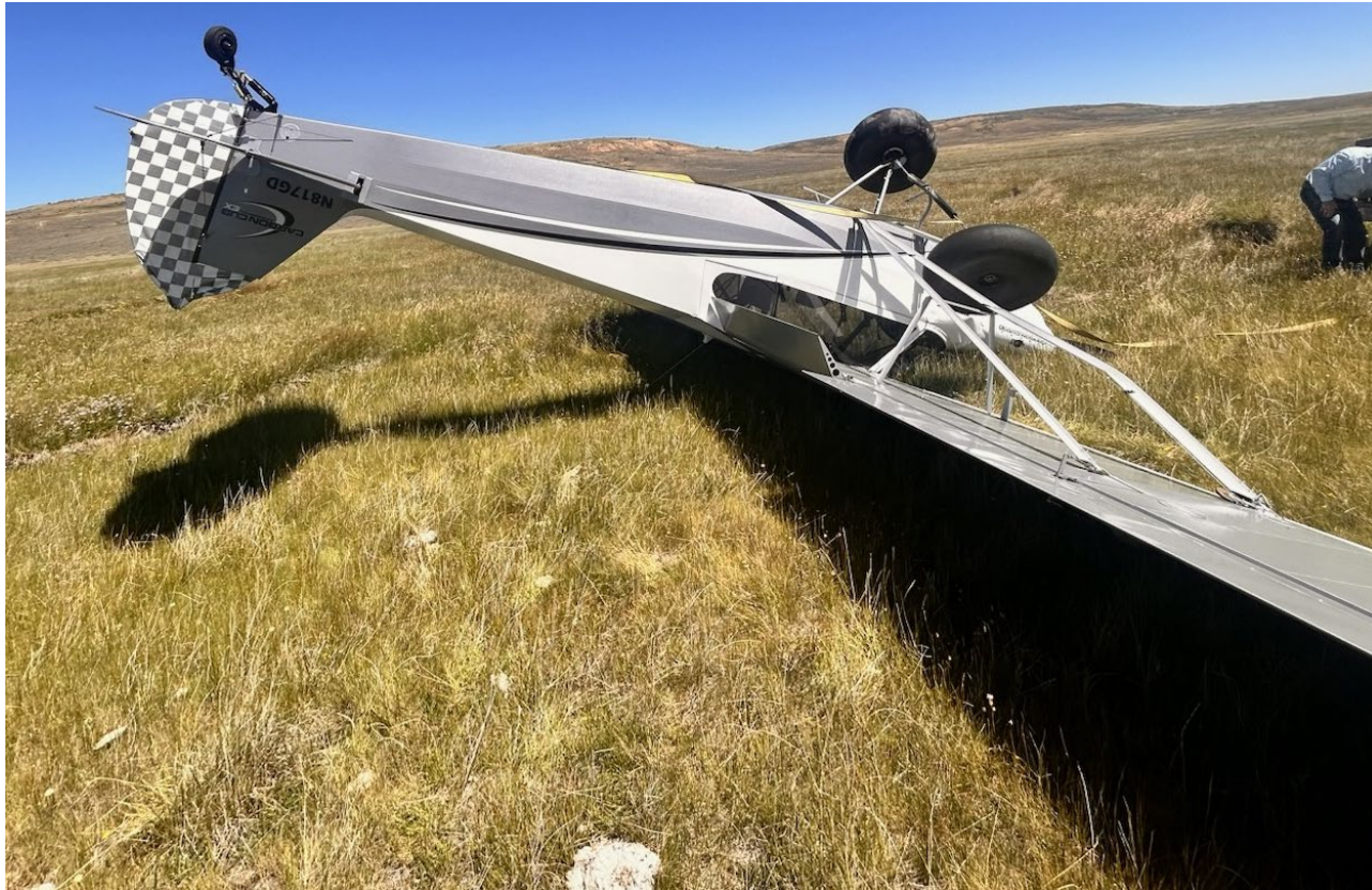
Photograph 1 - View of damage to the left wing lift strut and rudder (Courtesy of Pilot)
