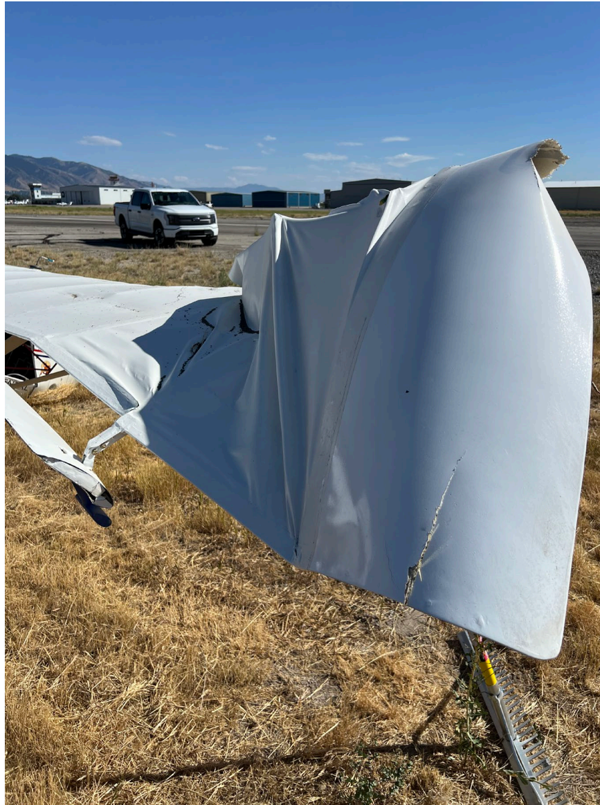
Photograph 1 - View of damage to right wing. (Courtesy of airport ops)
