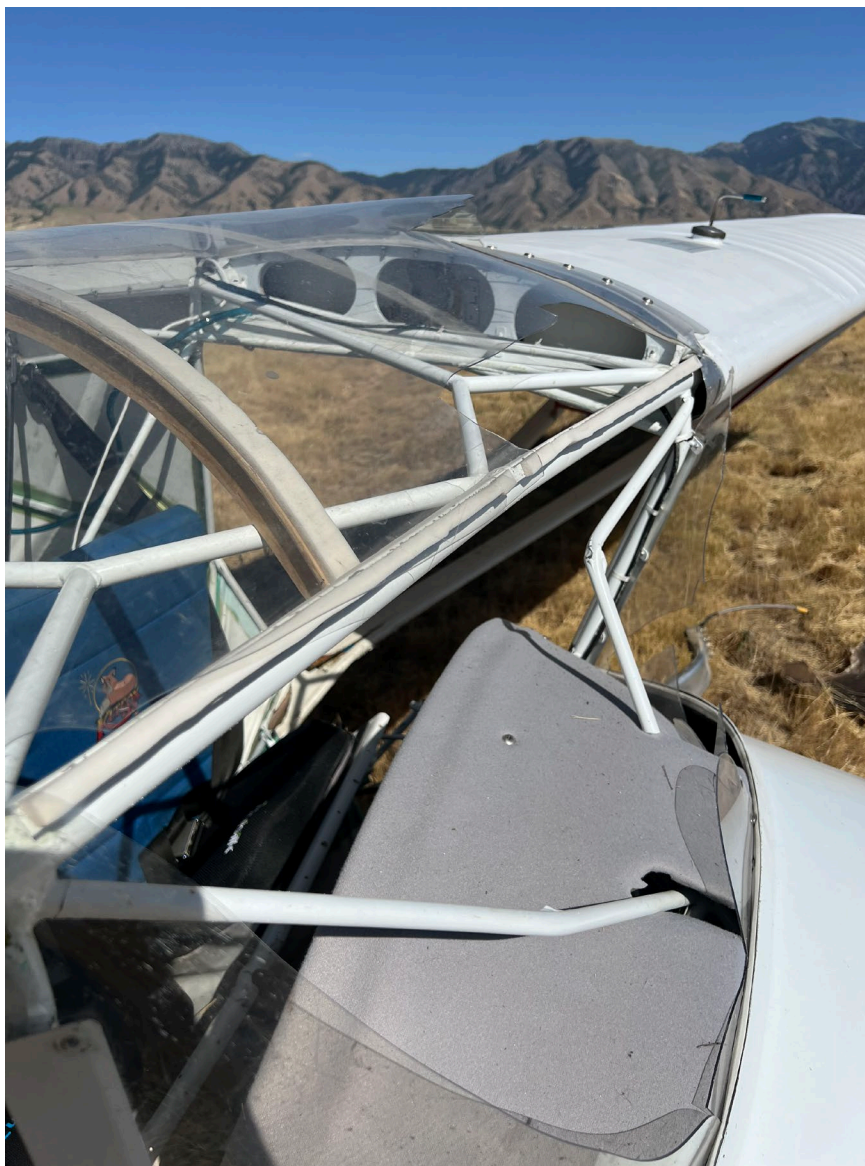
Photograph 2 - View of damage to forward fuselage. (Courtesy of airport ops)
