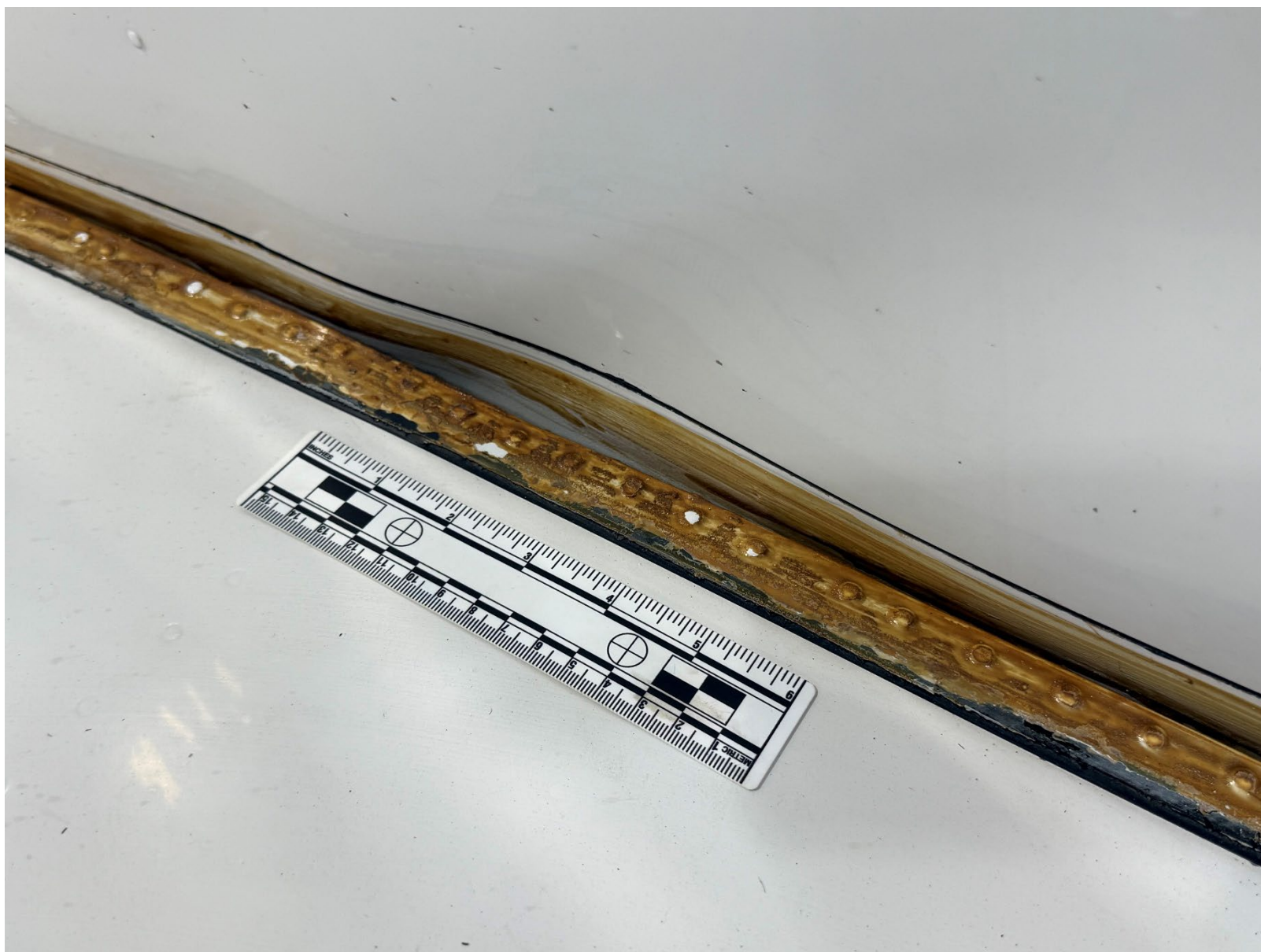
Photograph 2 - Airplane's left wing damage close-up as viewed from the left side. (Courtesy of FAA).
