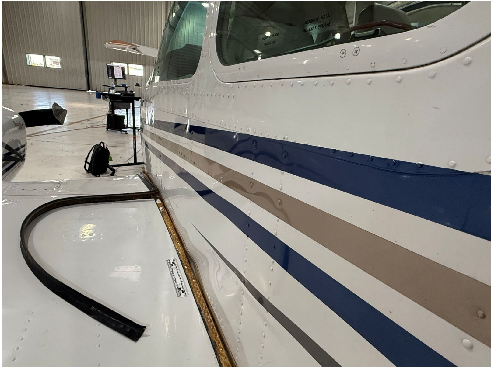
Photograph 1 - Airplane's left wing damage as viewed from the rear. (Courtesy of FAA).
