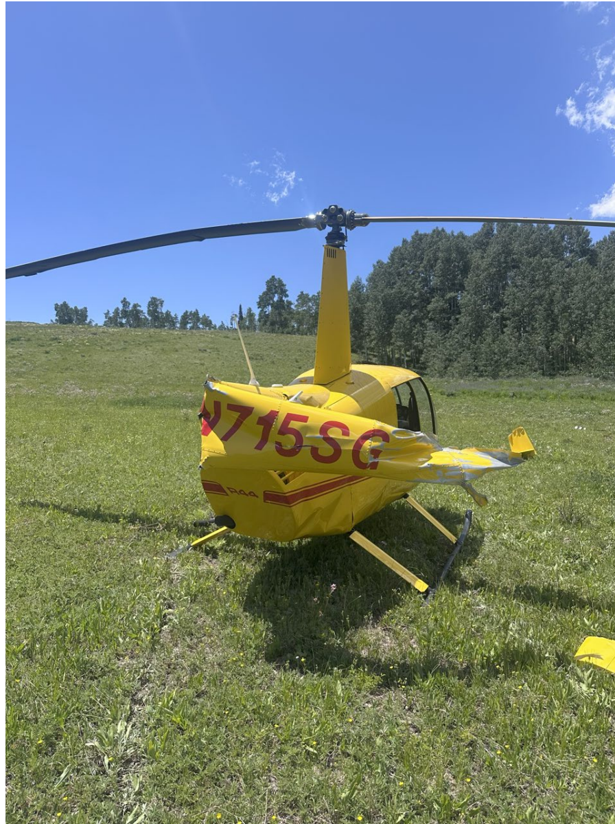
Photograph 1 - View tail damage (Courtesy of pilot)
