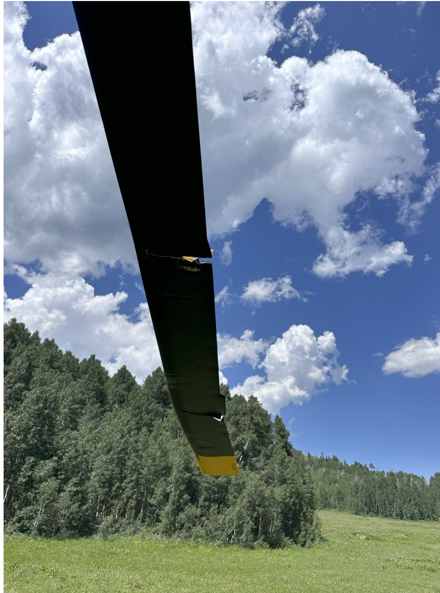
Photograph 2 - View of main rotor damage (Courtesy of Pilot)
