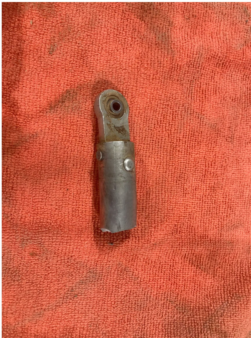
Photograph 3 - Fractured Steering Shaft (Courtesy of Pilot)
