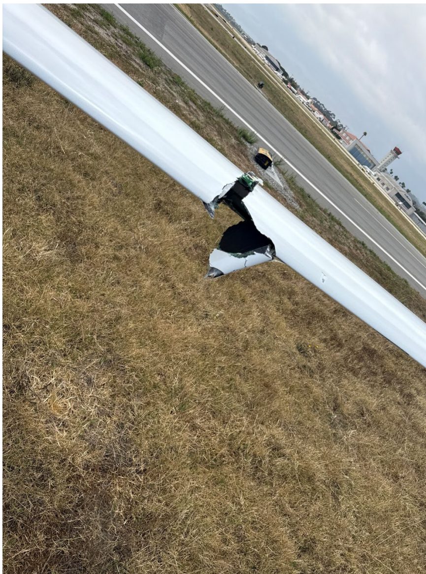
Photograph 1 - View of left-wing damage (Courtesy of airport operations)
