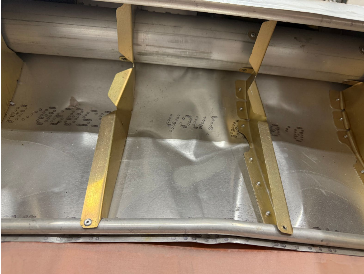
Photograph 2 - Top view of damage to right wing ribs (Courtesy of A&P)
