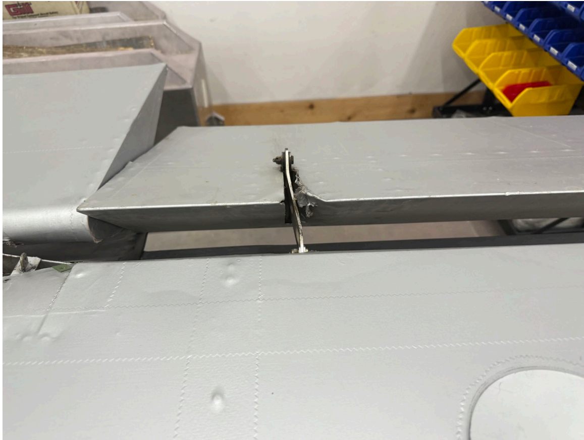
Photo 4 - View of damage to right aileron leading edge and attachment points (Courtesy of A&P)
