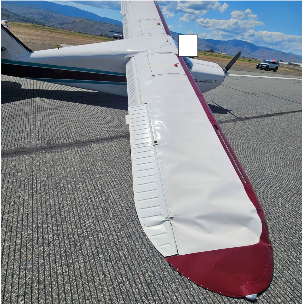
Photograph 1 - View of Damage to the Right Wing (Courtesy of the Pilot)
