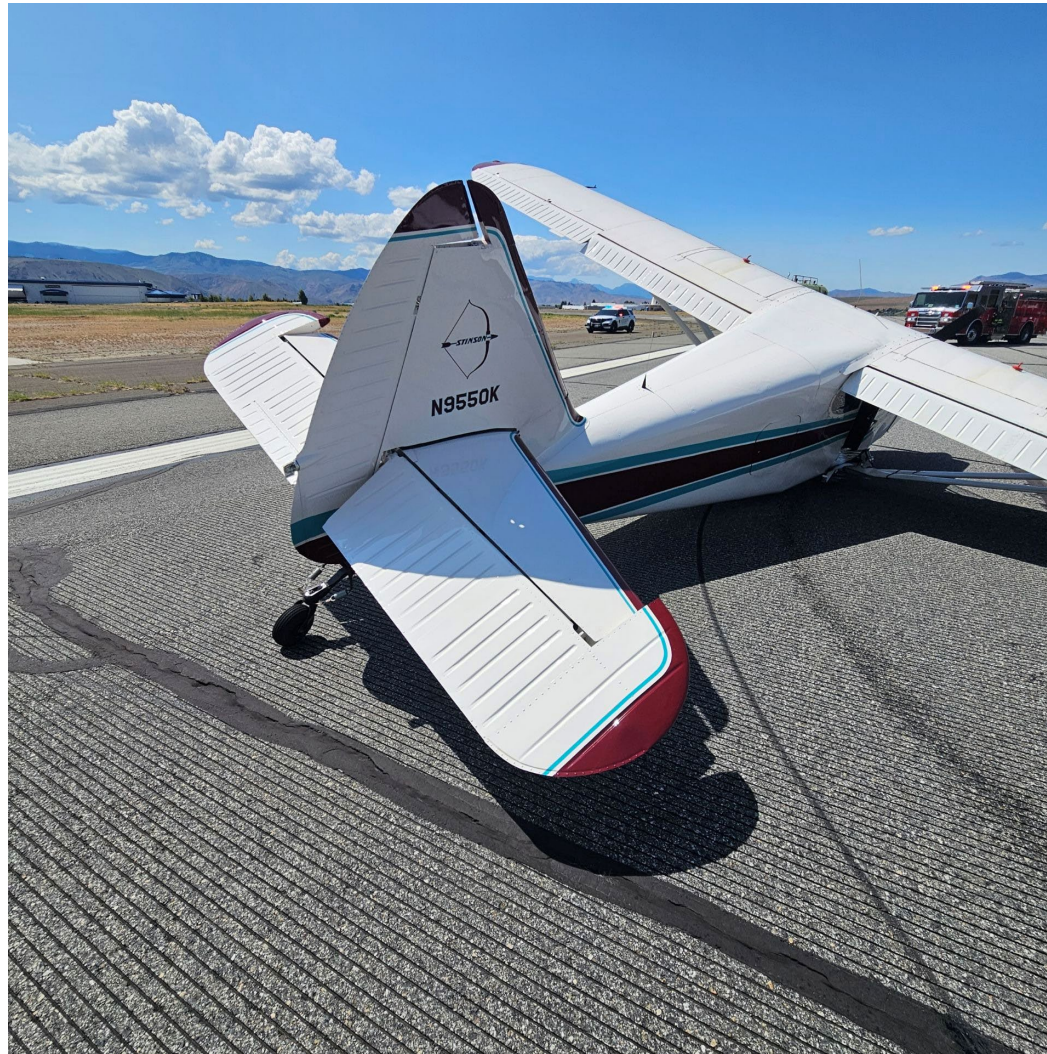
Photograph 2 - Right Side View of Airplane Note Fuselage Damage Aft of the Landing Gear (Courtesy of the Pilot)
