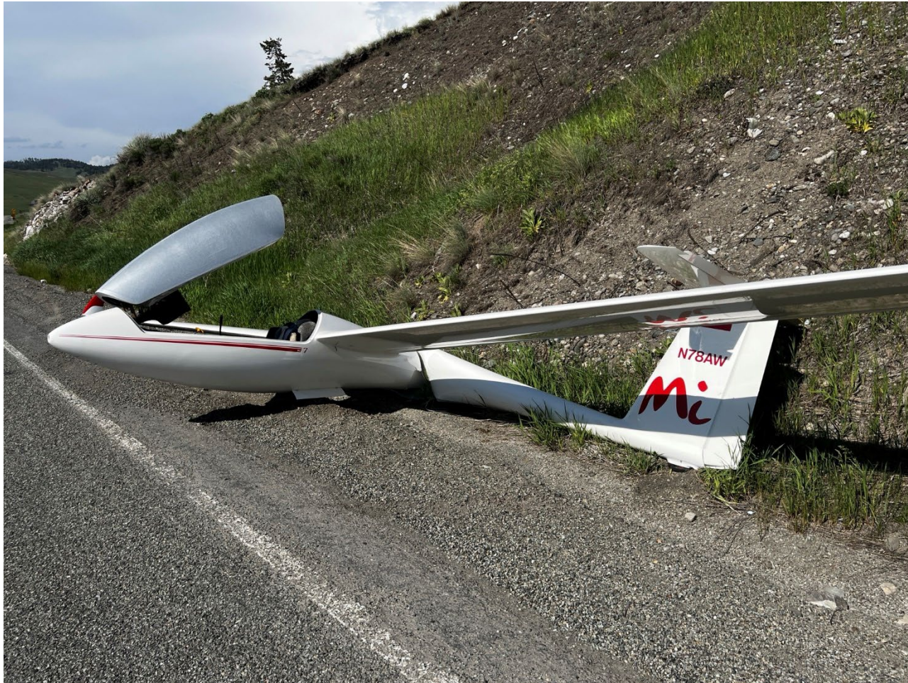
Photograph 1 - View of substantial damage to the aft fuselage (Courtesy of FAA)
