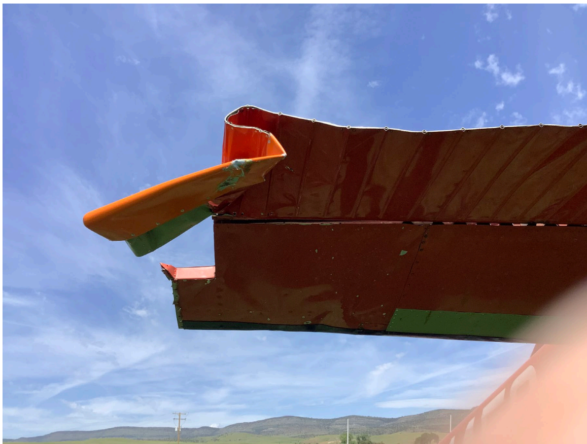
Photograph 1 - View of damage to elevator and horizontal stabilizer. (Courtesy of pilot)
