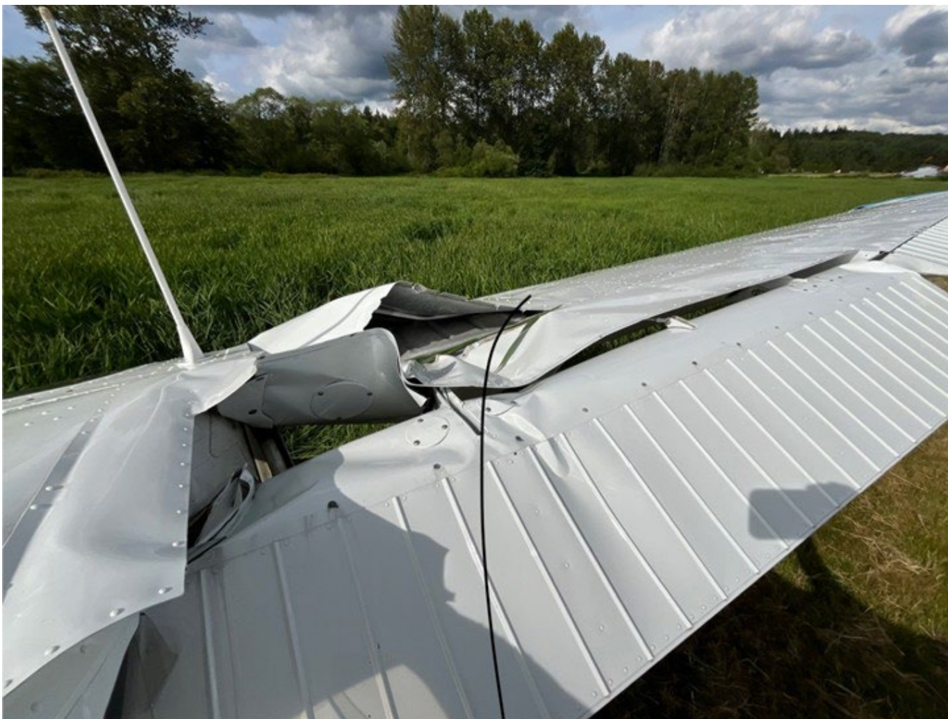
Photograph 2 - View of substantial damage to the right wing. (Courtesy of local law enforcement.)
