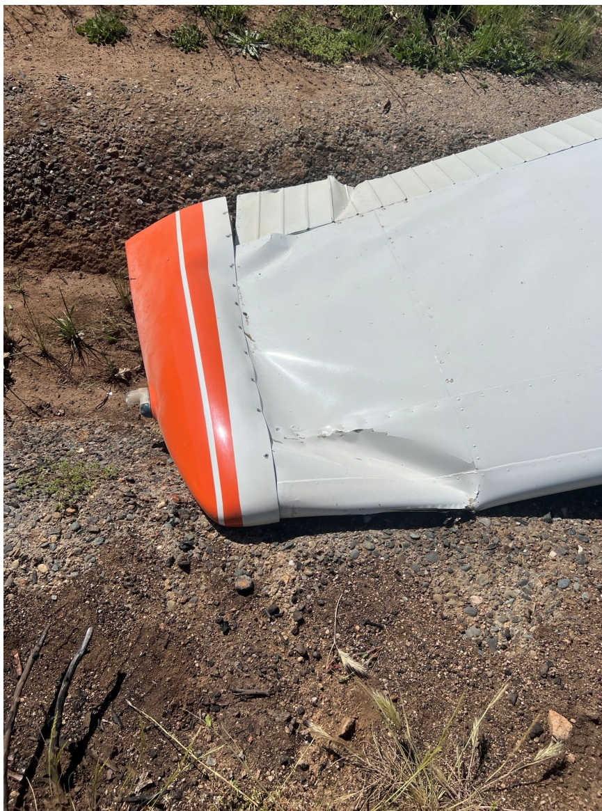
Photograph 3 - Right wing and aileron damage. (Courtesy of the pilot)
