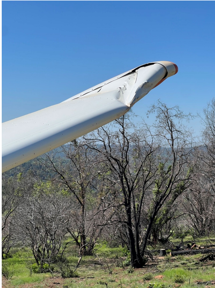
Photograph 2 - Left wing damage. (Courtesy of the pilot)
