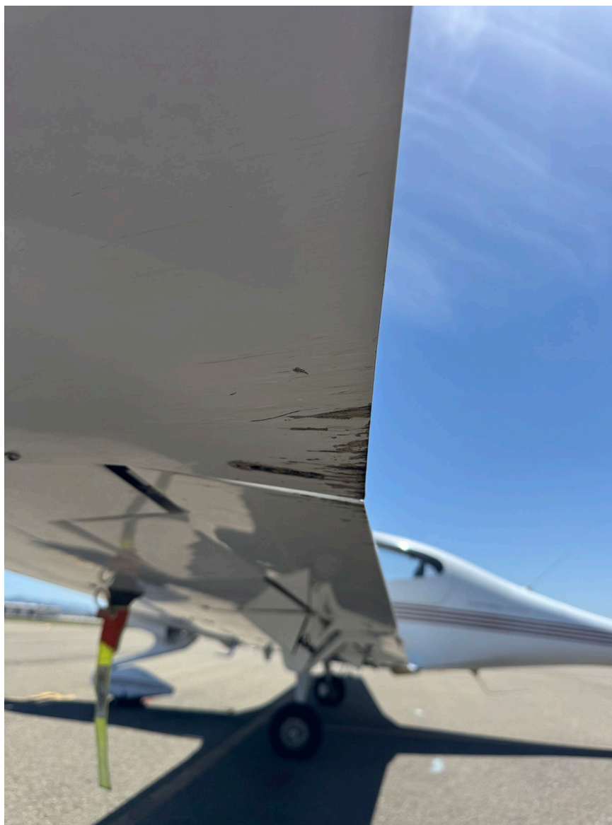
Photograph 2 - Left Wing Damage (Courtesy of Operator)
