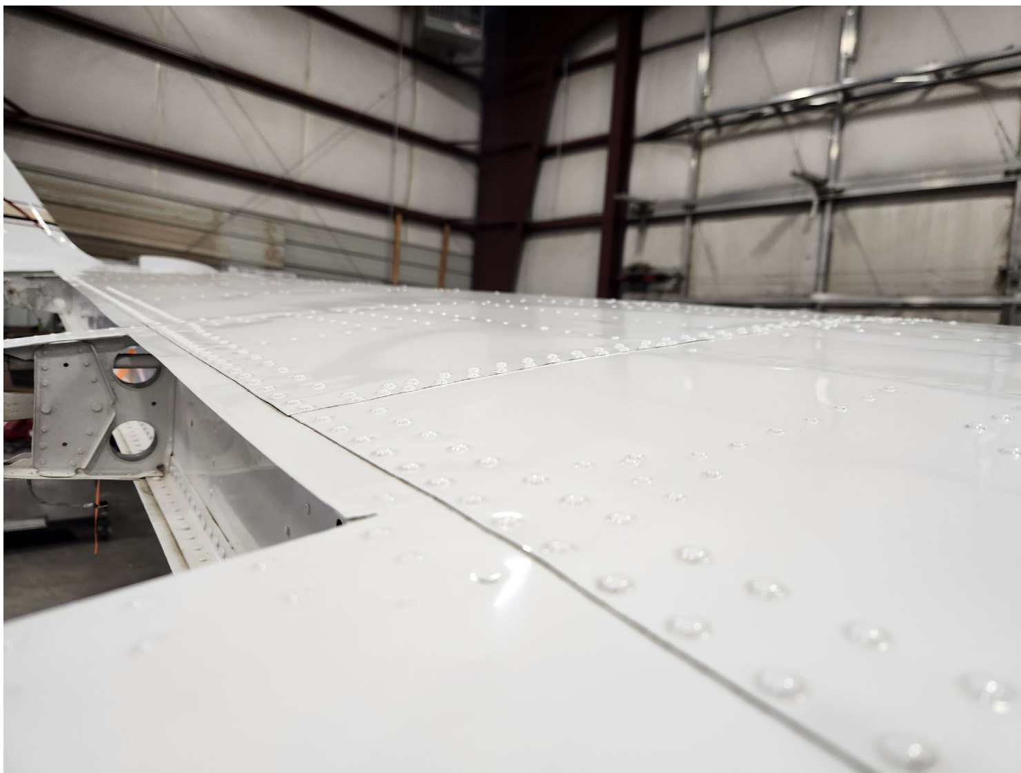
Photograph 2 - View of substantial damage in the form of deformation of left wing upper skins. (Courtesy of the FAA).
