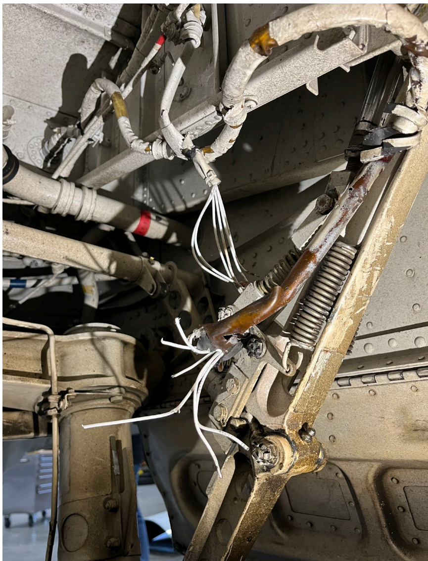
Photograph 3 - The broken wires in the left main landing gear down lock switch wire bundle. (Courtesy of the FAA).
