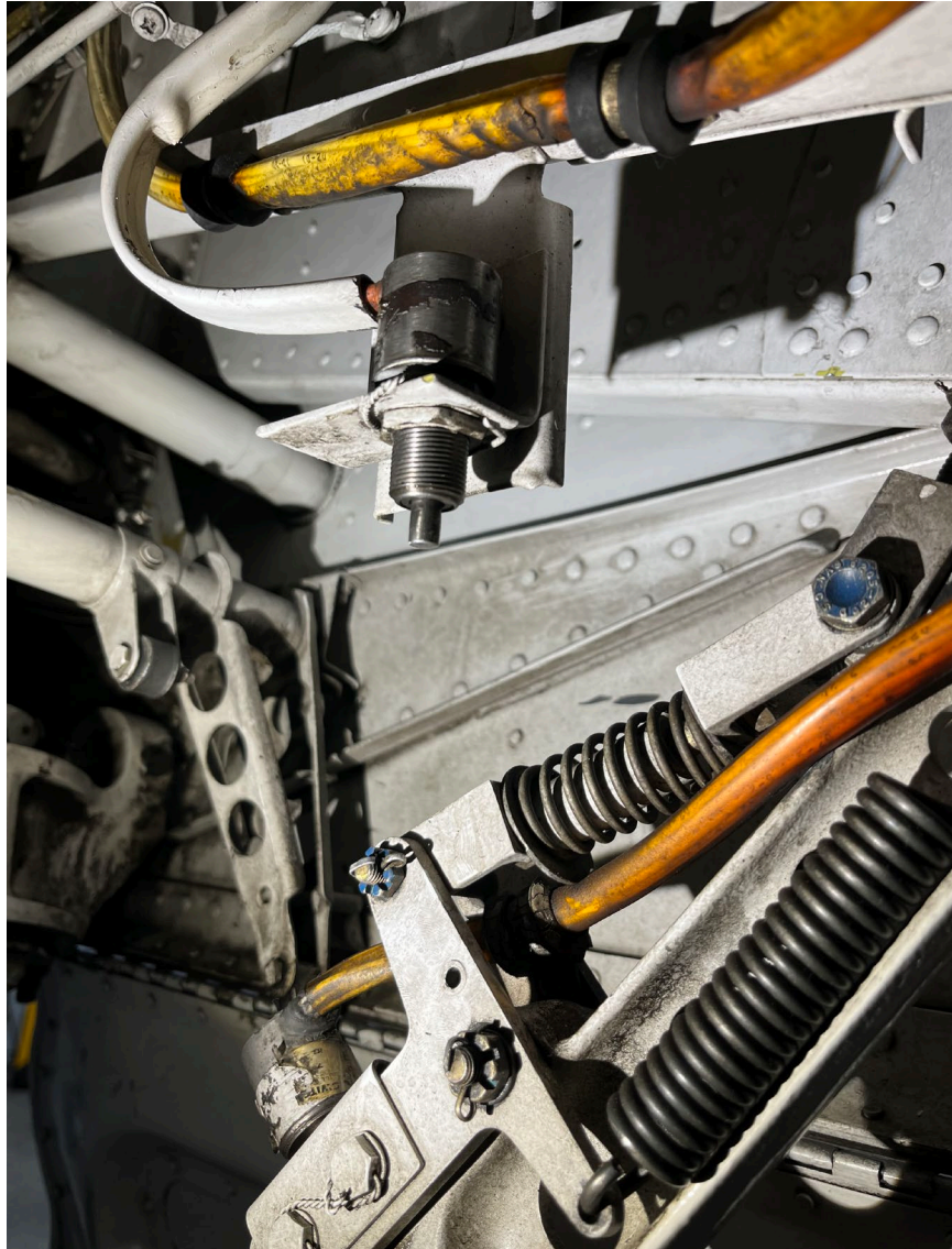
Photograph 4 - The landing gear up limit and downlock switches on a different Beech C90A. (Courtesy of the FAA).
