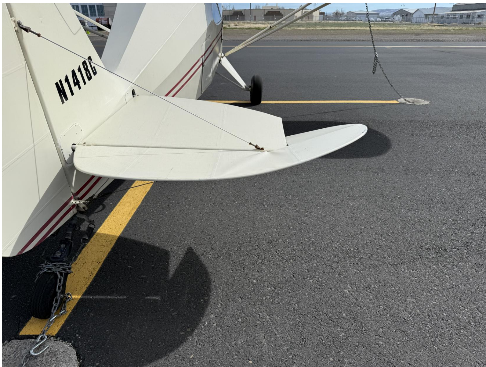
Photograph 4 - Accident airplane, right elevator damage. (Courtesy of the pilot)
