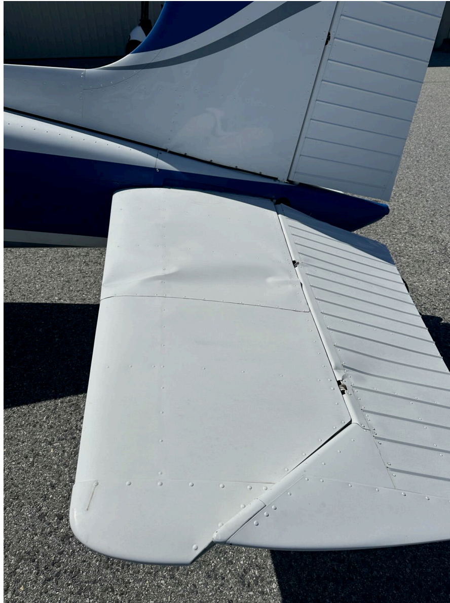
Photograph 3 - substantially damaged horizontal stabilizer (Courtesy of SQL Airport Operations)
