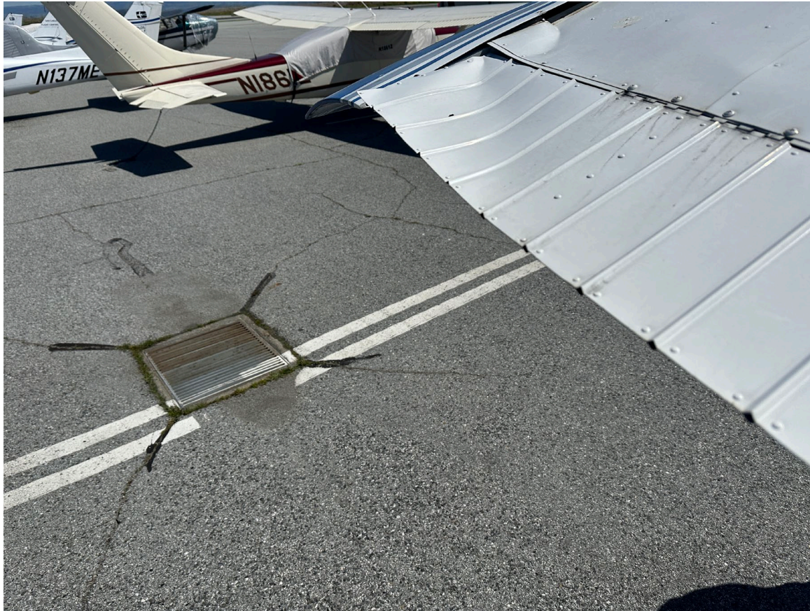
Photograph 2 - substantially damaged left wing and aileron (Courtesy of SQL Airport Operations)
