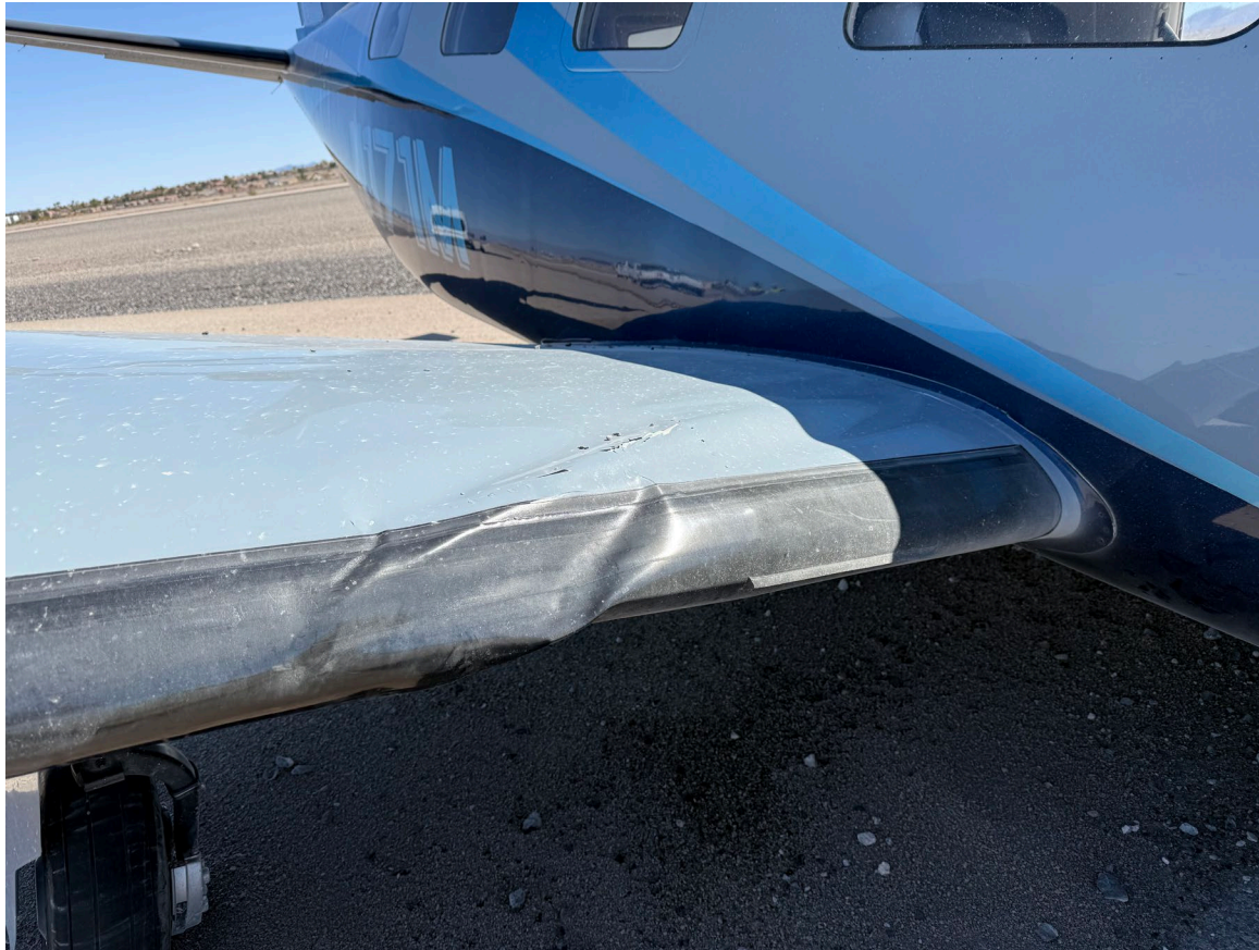
Photograph 2 - Right wing damage. (Source airport manager)
