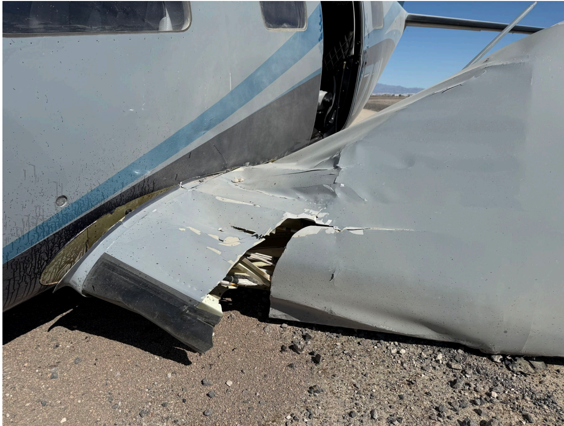
Photograph 3 - Left wing damage. (Source airport manager)
