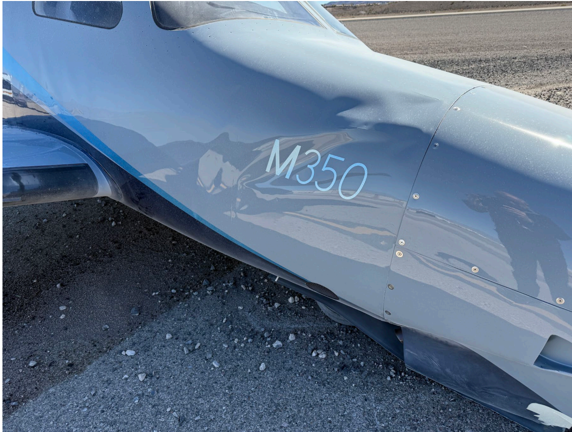
Photograph 1 - N171M, Fuselage damage. (Source airport manager)
