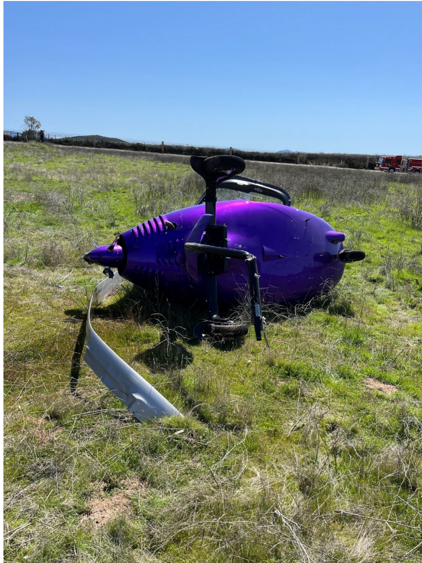
Photograph 1 - View of damage to keel and main rotor blade (Courtesy of LEO)
