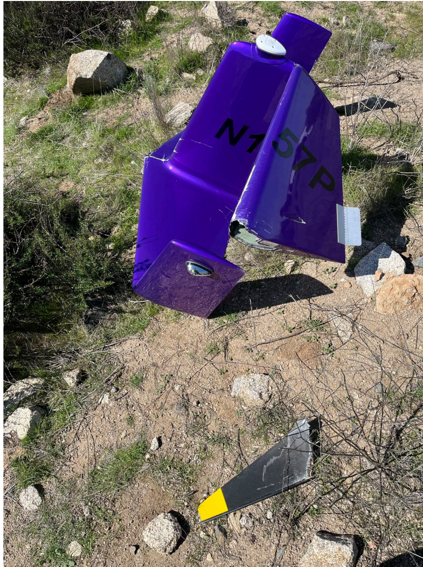
Photograph 2 - View of damage to the rudder (Courtesy of LEO)
