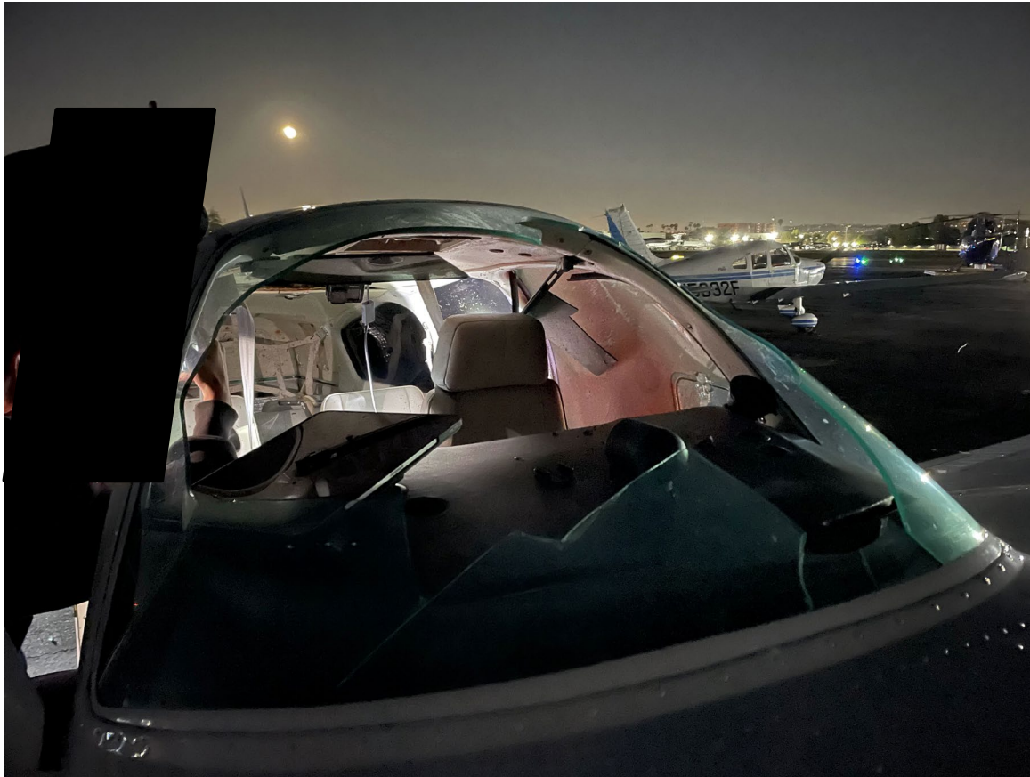
Photograph 1 - Forward View of Broken Windshield (Courtesy of Airport Operations)
