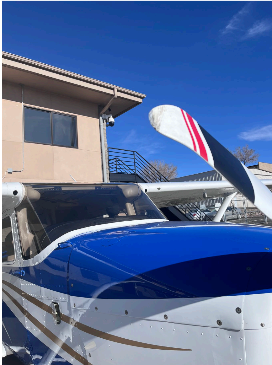
Photograph 1 - Propeller blade damage (Courtesy of ERAU)
