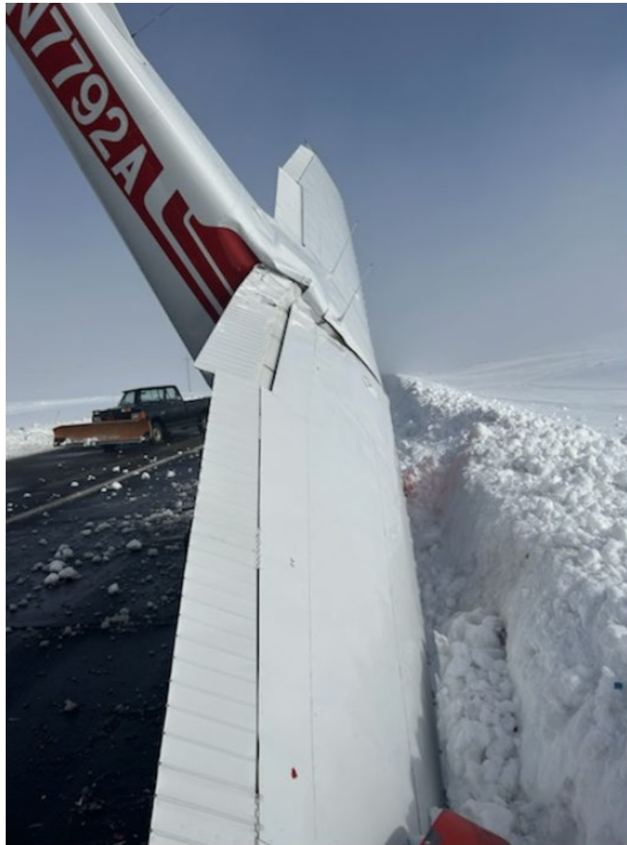
Photograph 2 - Top view of right-wing damage (Photo Courtesy of pilot)
