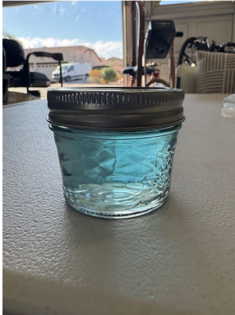
Photograph 3 - The fuel recovered from the right fuel tank (Courtesy of the FAA)
