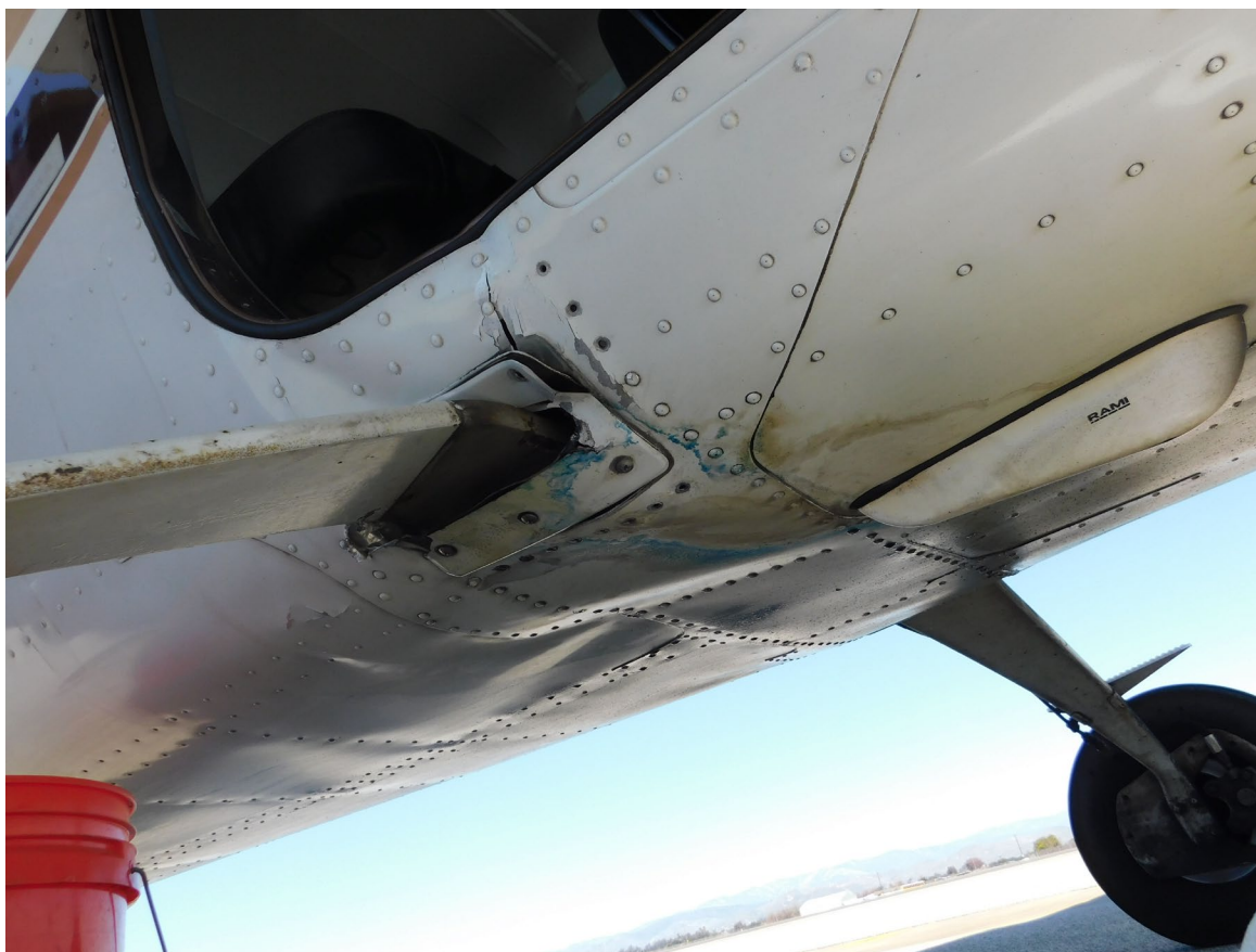
Photograph 2 - View of substantial damage to fuselage (Courtesy of the FAA)
