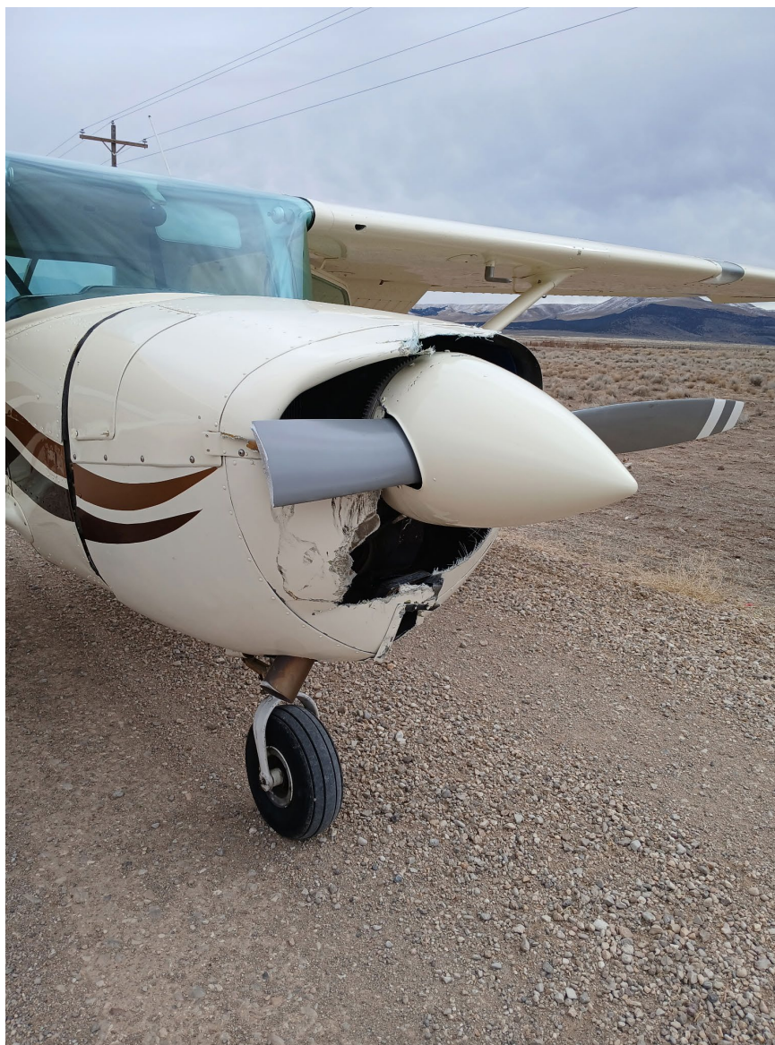
Photograph 3 - A view of the fractured propeller blade. (Courtesy of the pilot.)
