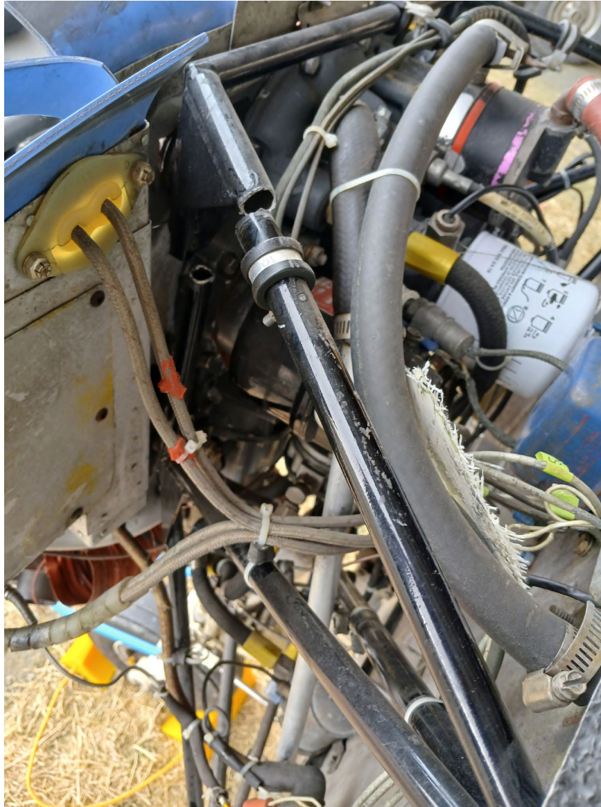
Photograph 4 - A view of the substantial damage to the engine mount. (Courtesy of the pilot.)
