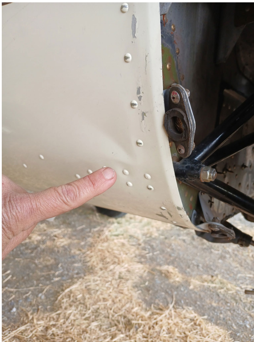
Photograph 5 - A view of the substantial damage to the fuselage. (Courtesy of the pilot.)
