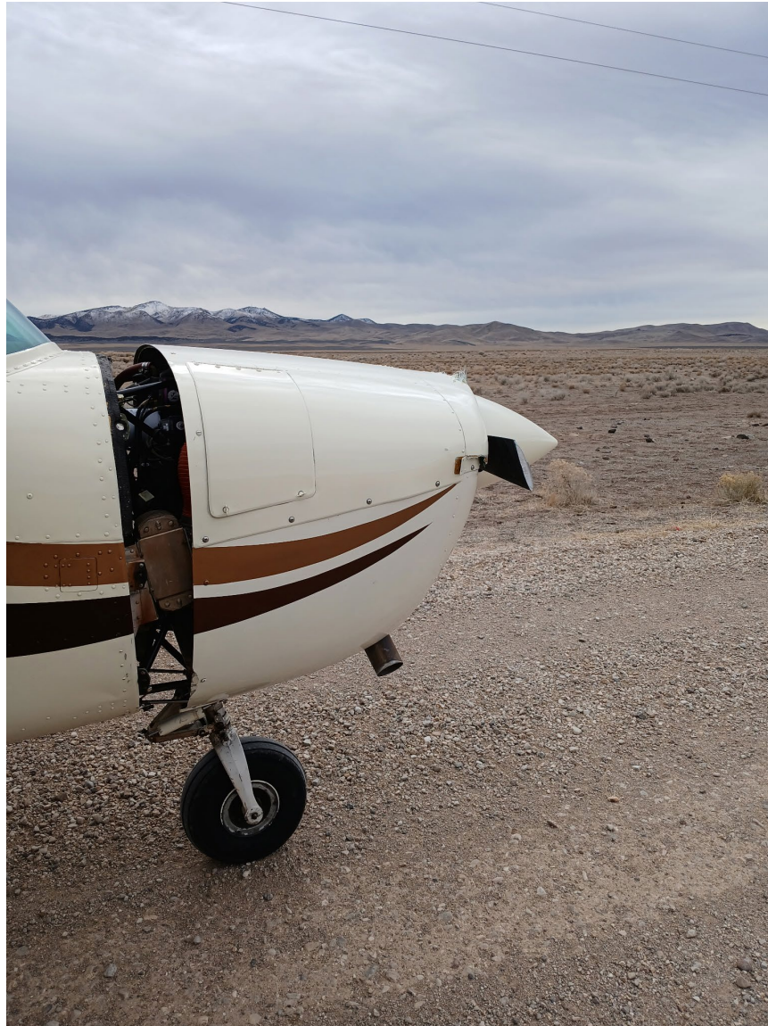
Photograph 2 - A view of the fractured propeller blade and damaged engine cowlings. (Courtesy of the pilot.)
