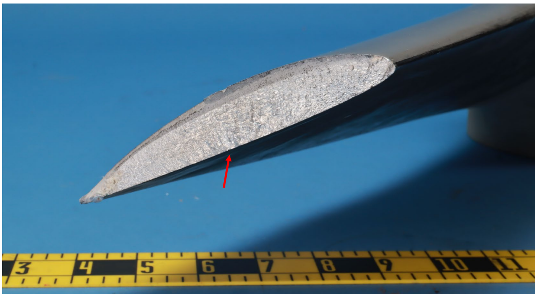
Figure 2. Fracture surface exhibiting a flat fracture and shear lip along the blade back. Fracture origin indicated by the red arrow.
