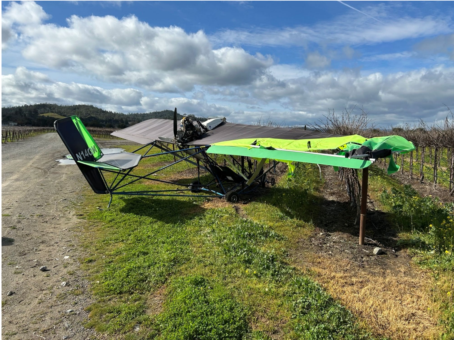
Photograph 1 View of Airplane with Damaged Wing in Vineyard (Courtesy of Local Law Enforcement)
