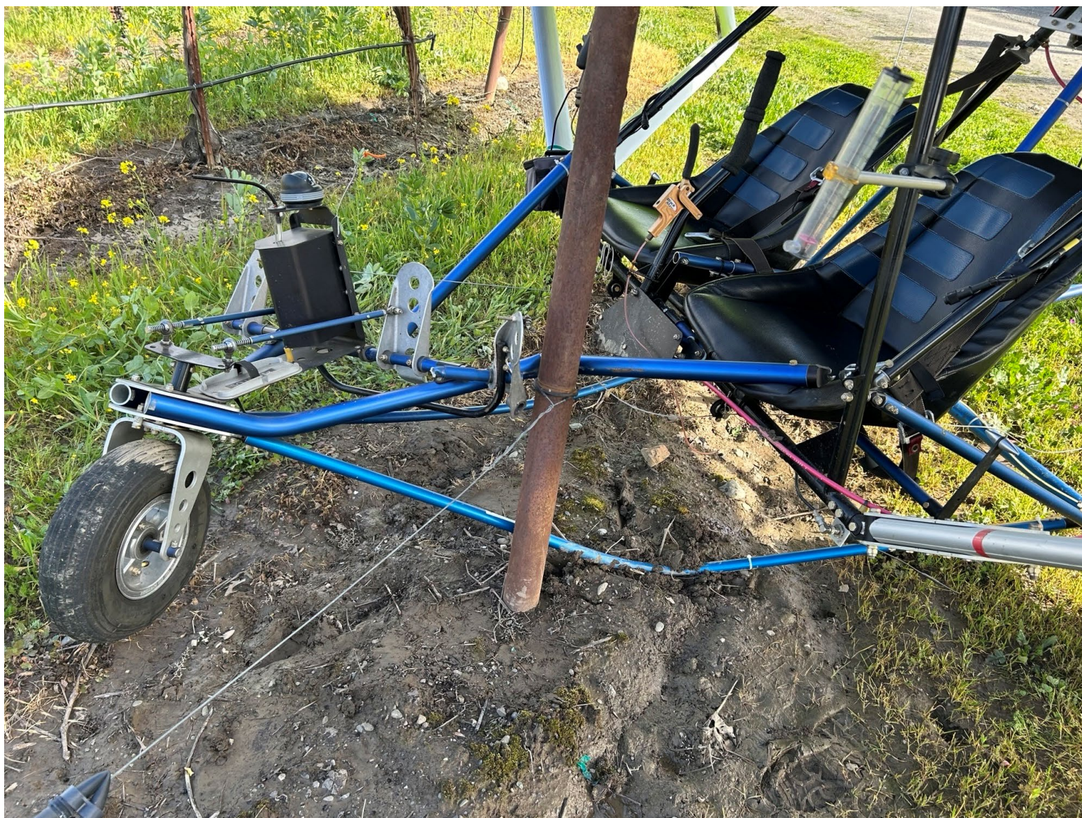
Photograph 2 - Substantially Damaged Fuselage (Courtesy of Local Law Enforcement)
