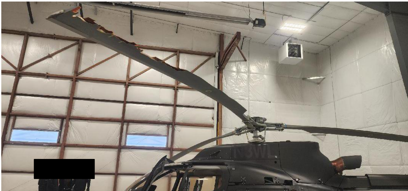
Photograph 5 - Helicopter main rotor blade damage. (Courtesy of the FAA)
