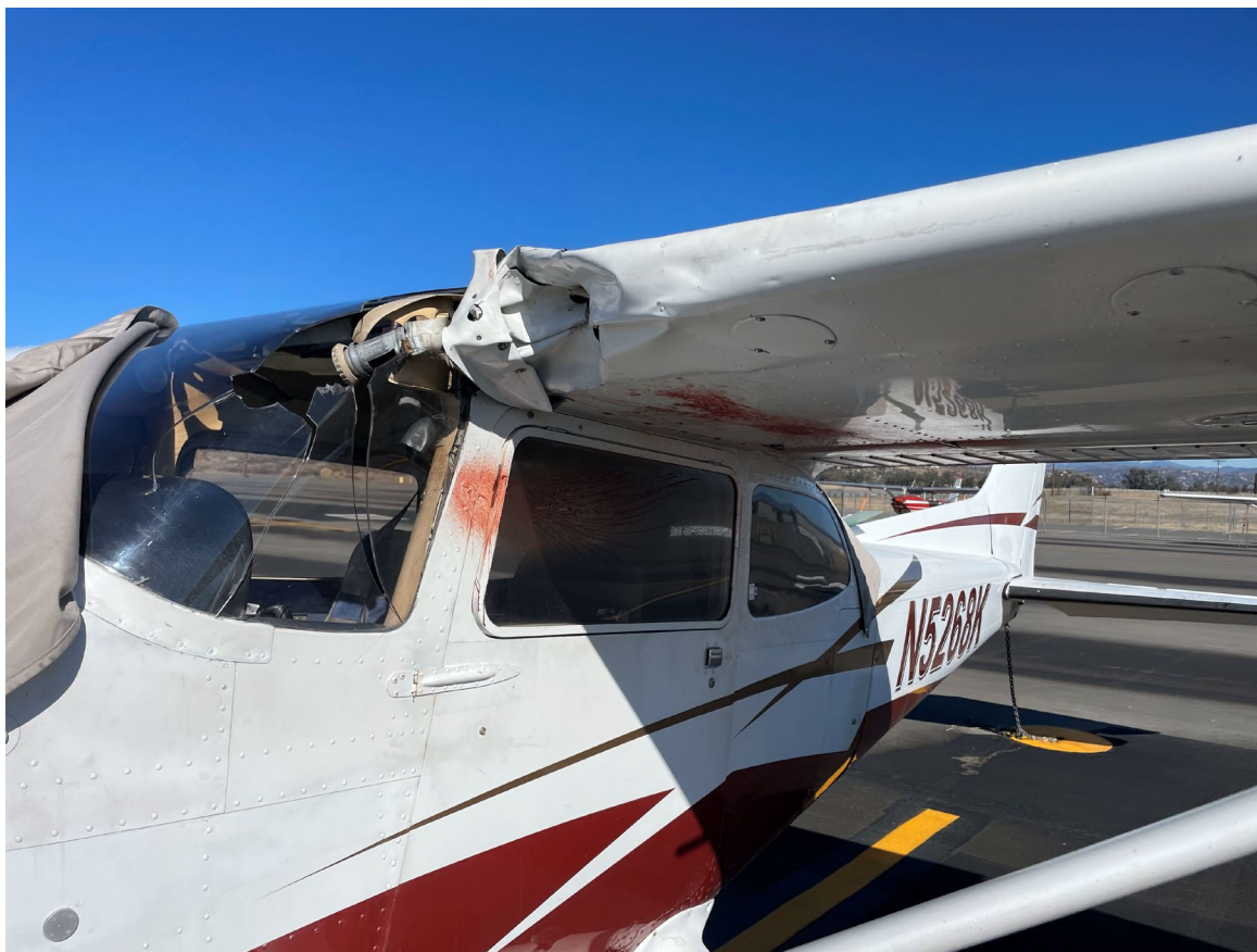
Photograph 1 - N5268K, showing substantial damage to the left wing. Source airport operations.
