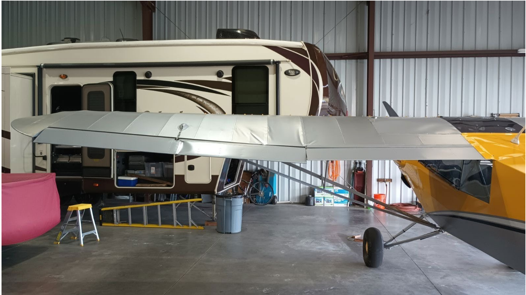
Photograph 1 - Airplane's left wing damage as viewed from the rear. (Courtesy of Airplane Owner).
