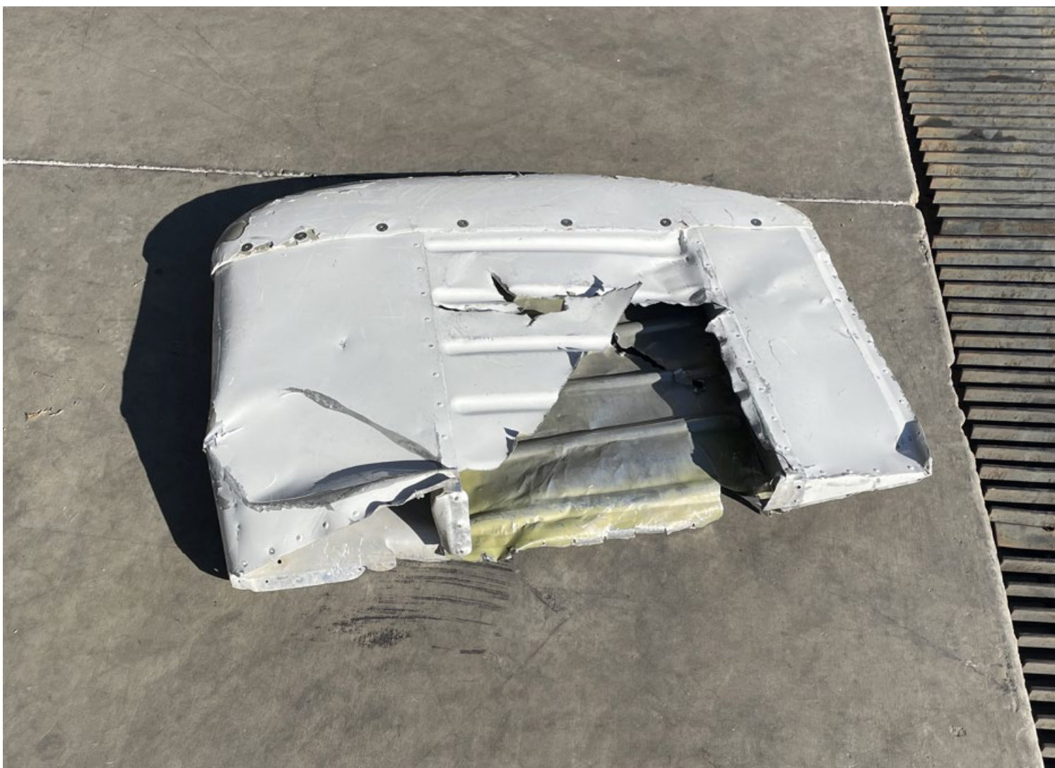
Photograph 5 - Right stabilator end cap after second retrieval
