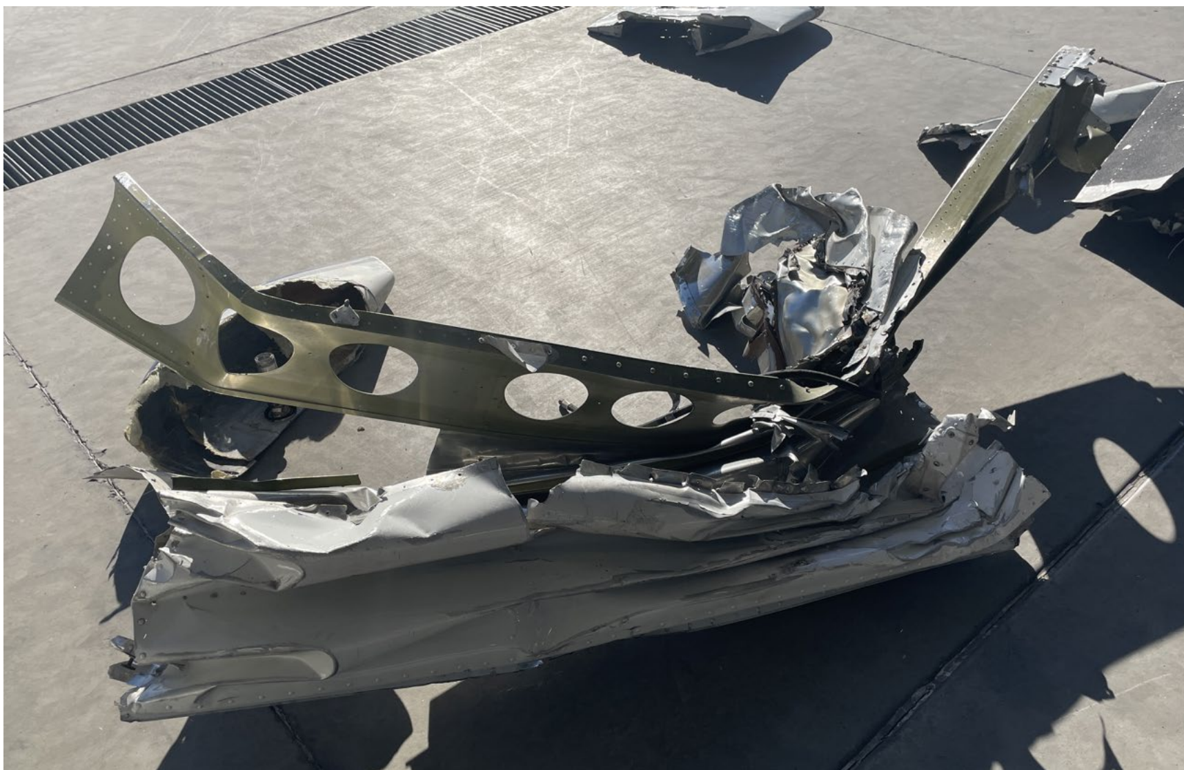
Photograph 7 - Midspan right wing after followup retrieval
