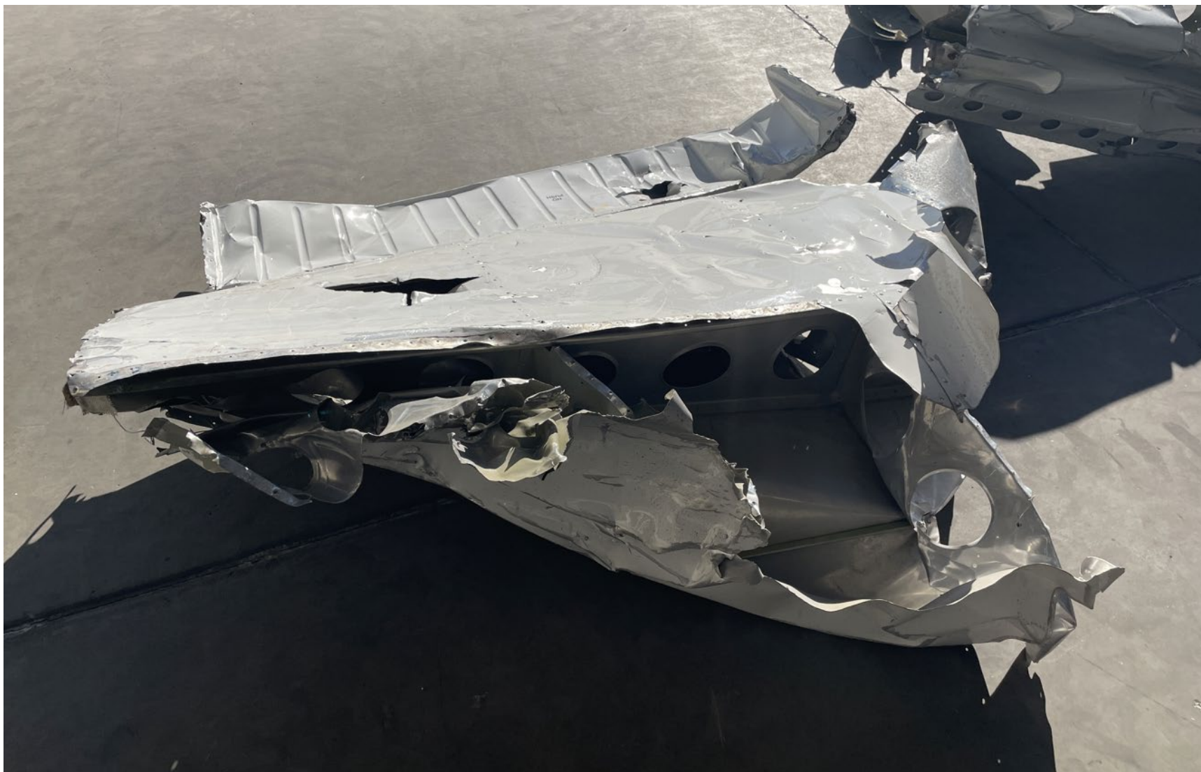
Photograph 6 - Inboard right wing section after followup retrieval
