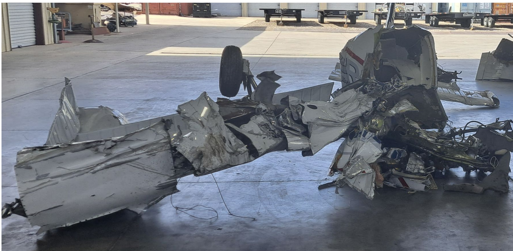
Photograph 3 - Left wing and fuselage during initial layout (Courtesy of Piper Aircraft Company)
