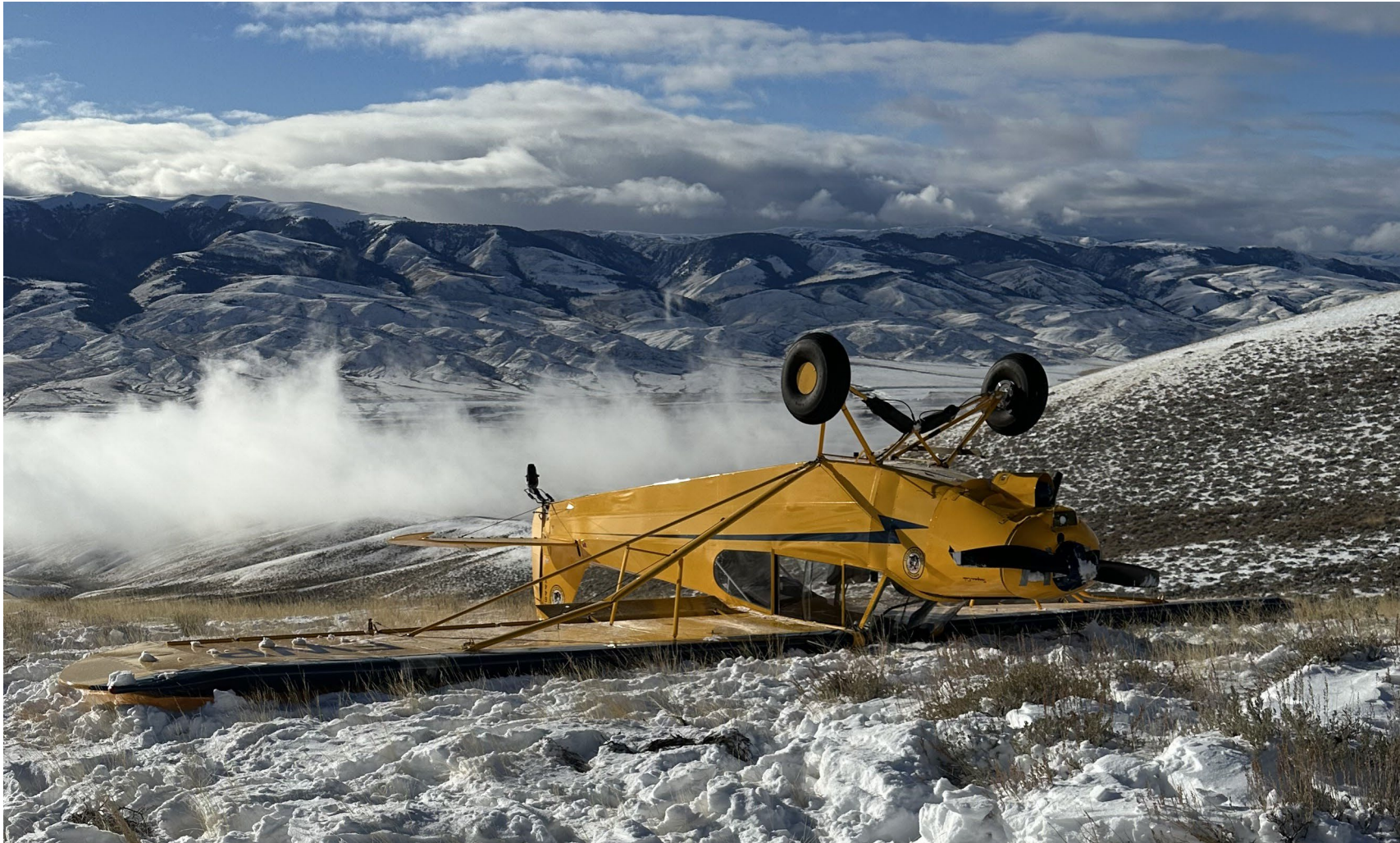
Photograph 1 - View of wing and strut damage (Courtesy of pilot)
