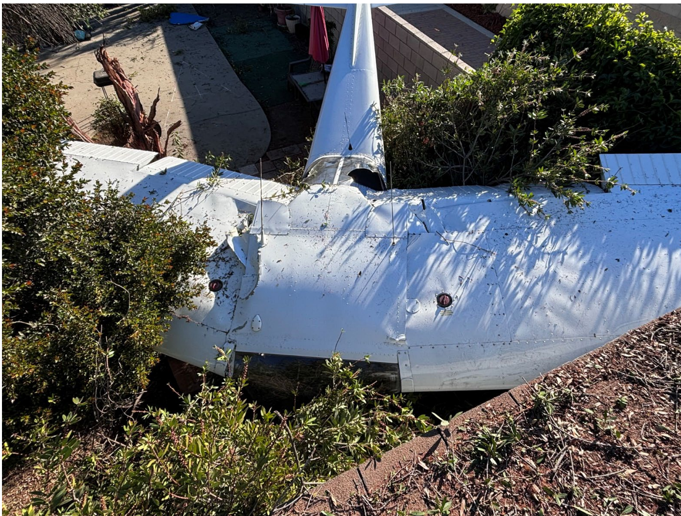
Photograph 2 - Top view of substantial damage to both wings (Courtesy of FAA)
