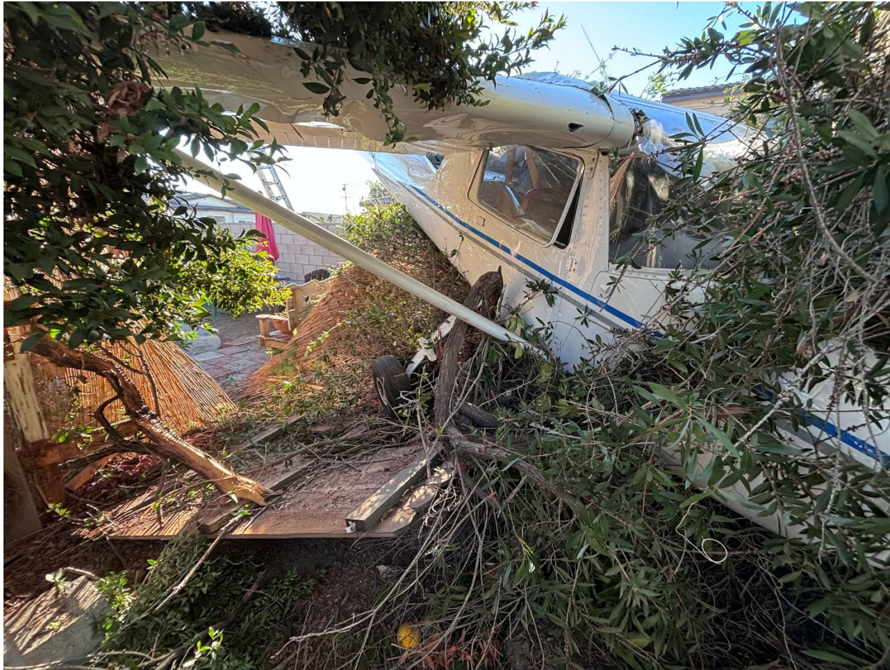
Photograph 1 - View of substantial damage to the right wing (Courtesy of FAA)
