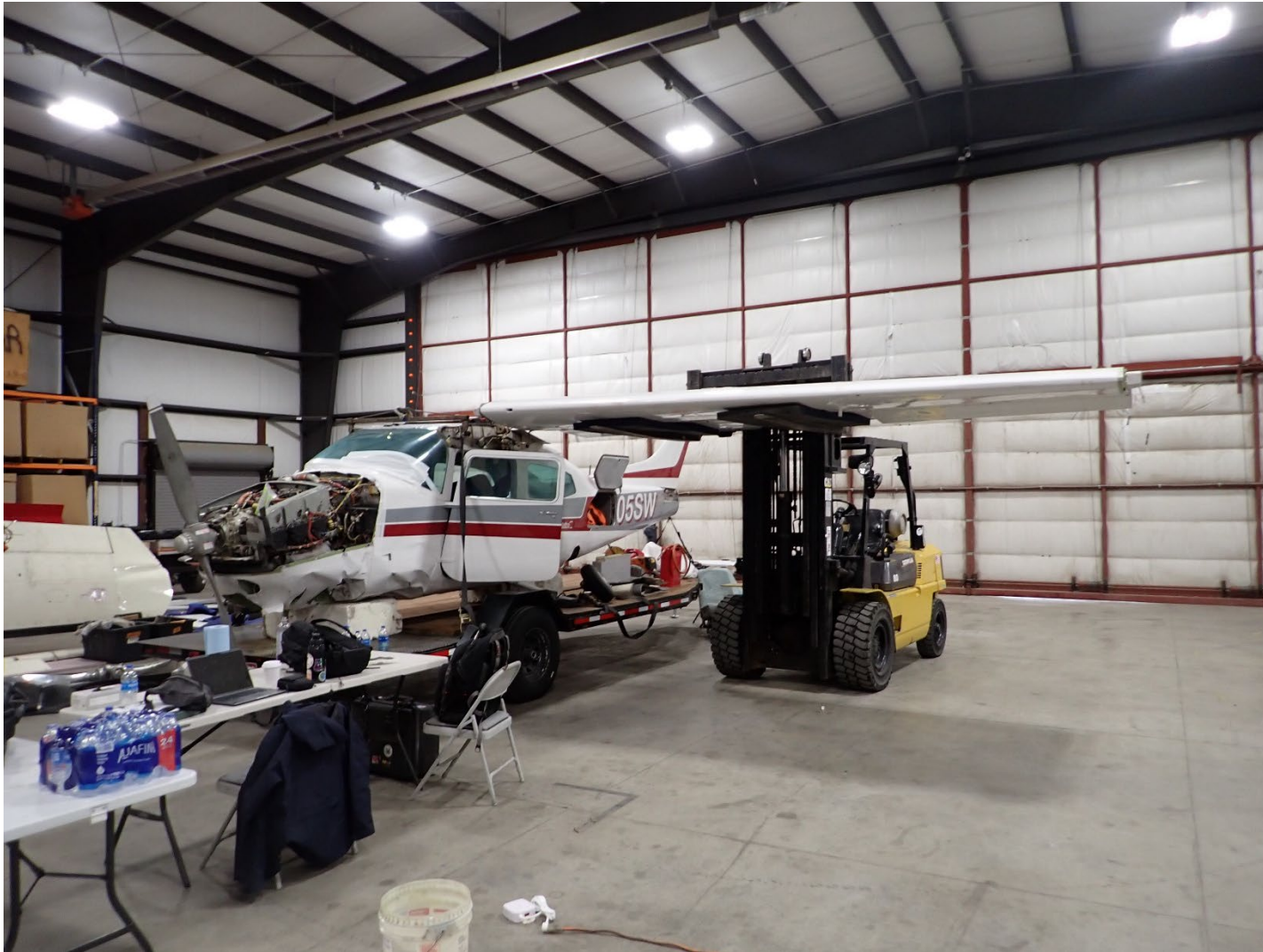
Photograph 4 - Airplane during testing of fuel quantity indicating system.
