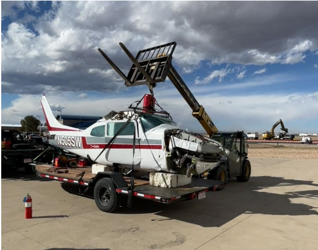
Fig 3: The airplane mounted on a trailer with the engine running.
