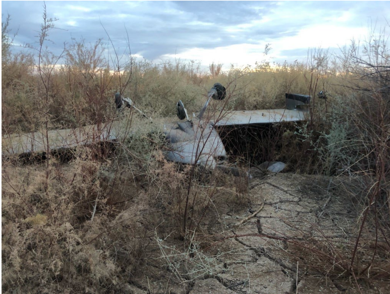
Photograph 1 - View of inverted airplane with substantial damage to the right wing (Courtesy of Pilot)
