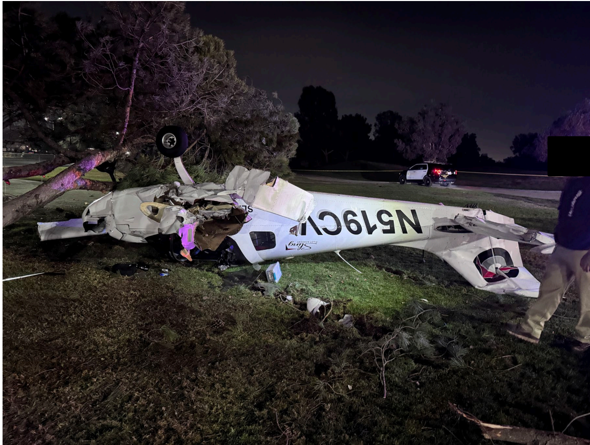
Photograph 3 - Substantial damage to the fuselage, left wing, left horizontal stabilizer, and elevator. (Courtesy of the operator)
