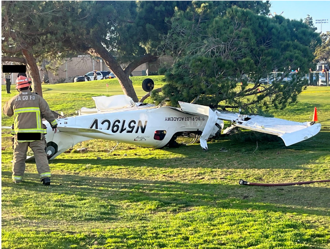
Photograph 2 - Substantial damage to the right wing, vertical stabilizer, and rudder. (Courtesy of the operator)
