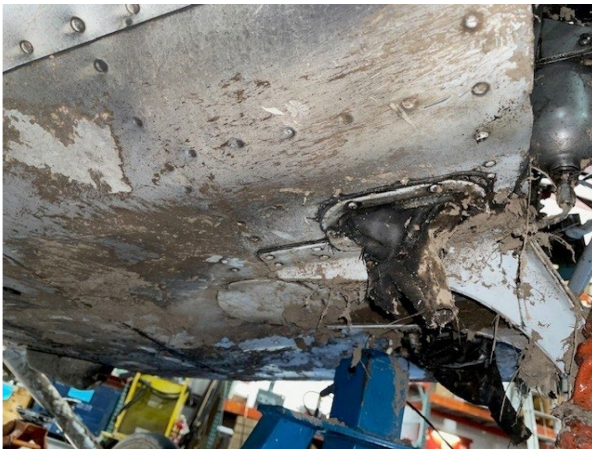
Photograph 4 - View of substantial damage to lower forward fuselage. (Courtesy of the FAA)
