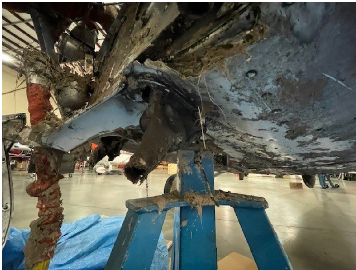
Photograph 3 - View of substantial damage to lower forward fuselage. (Courtesy of the FAA)
