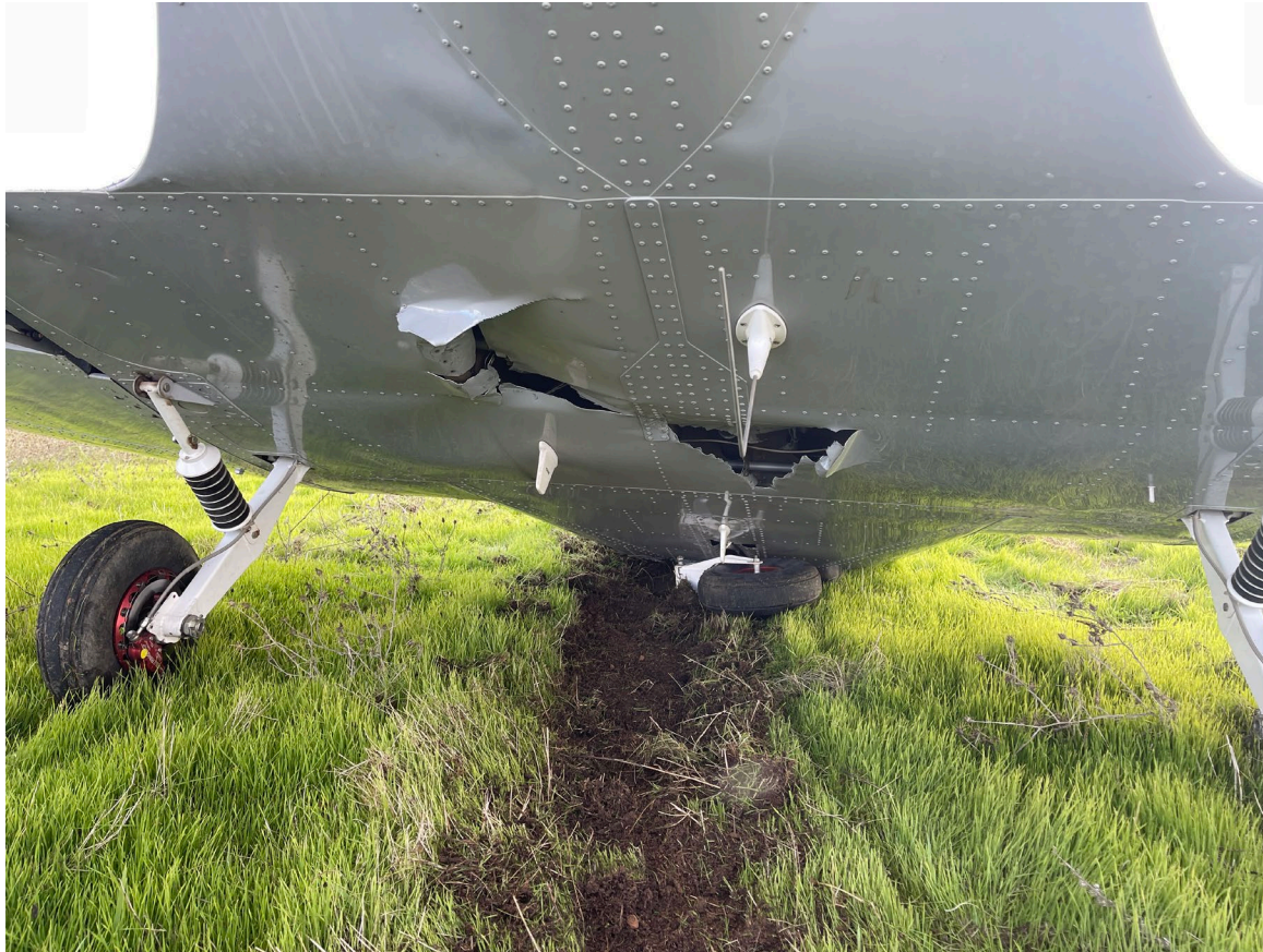
Photograph 2 - Lower fuselage damage. (Courtesy of FAA)
