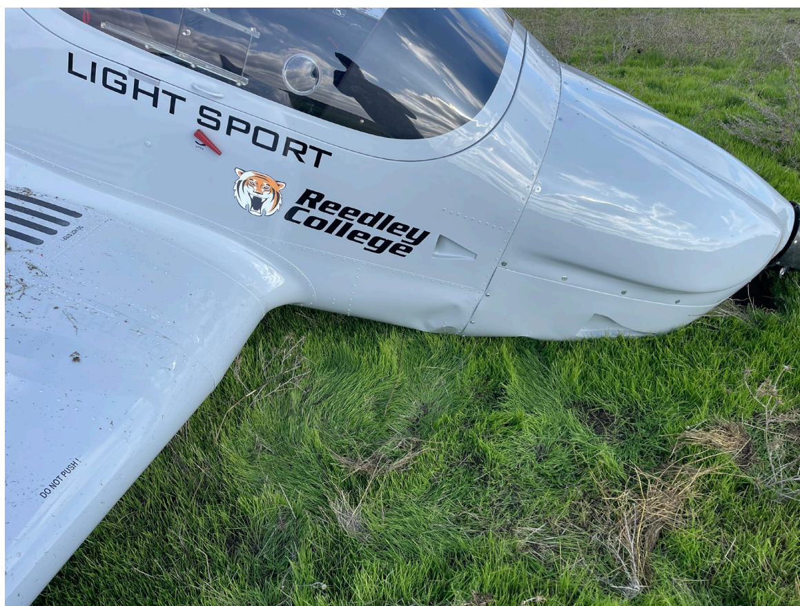
Photograph 1 - Forward lower fuselage damage. (Courtesy of FAA)
