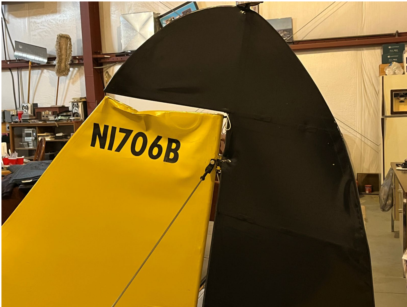
Photograph 2 - View of substantial damage to vertical stabilizer. (Courtesy of the FAA.)
