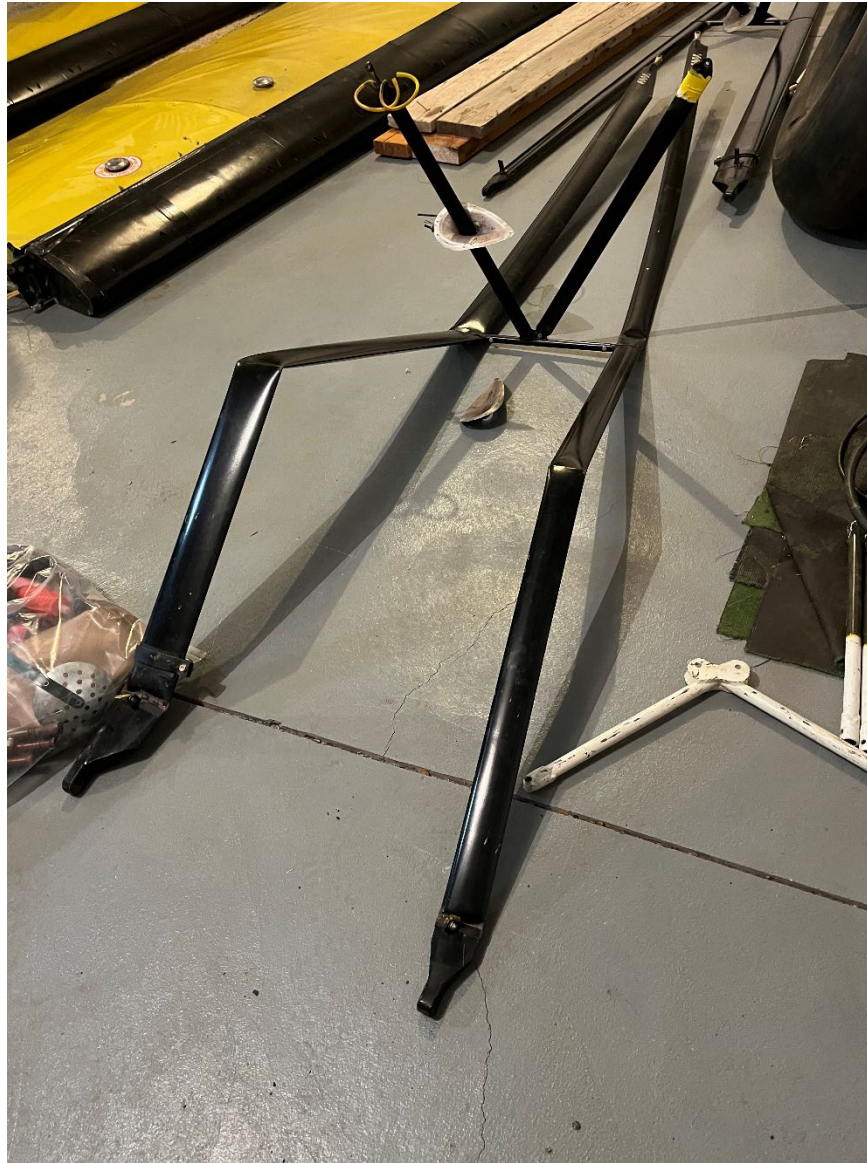
Photograph 3 - View of substantial damage to wing strut. (Courtesy of the FAA.)
