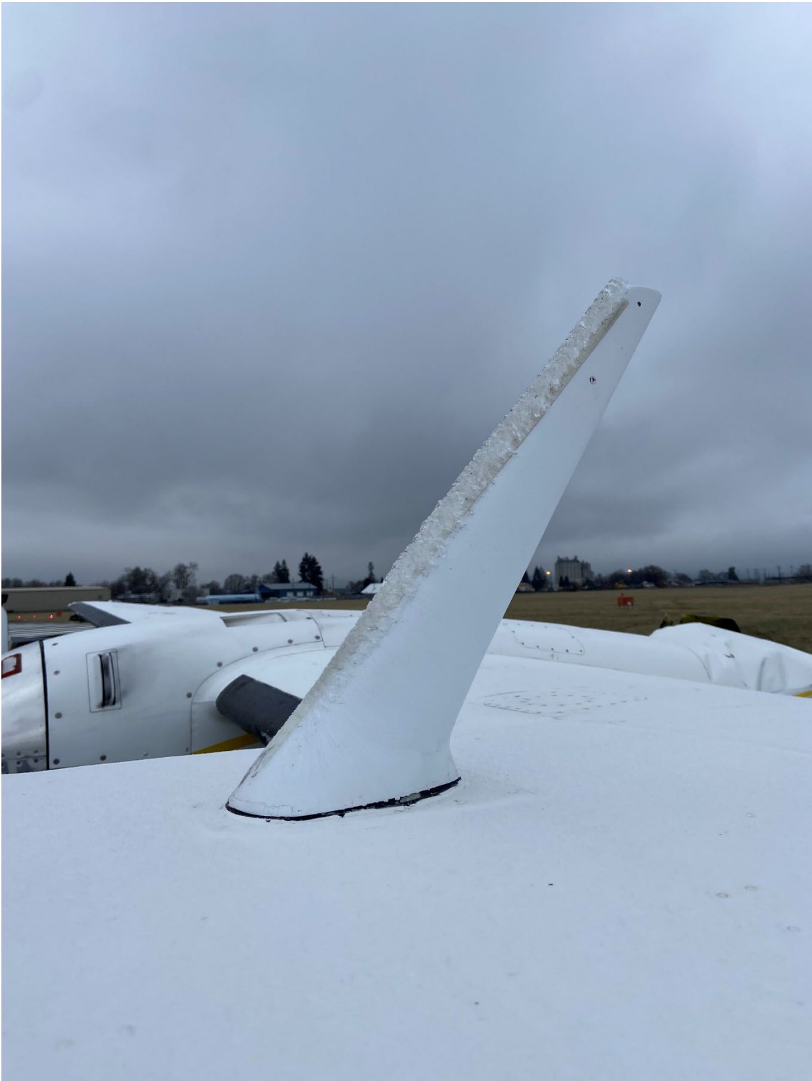
Figure 4: View of ice on fuselage antennas. (Courtesy of FAA)
