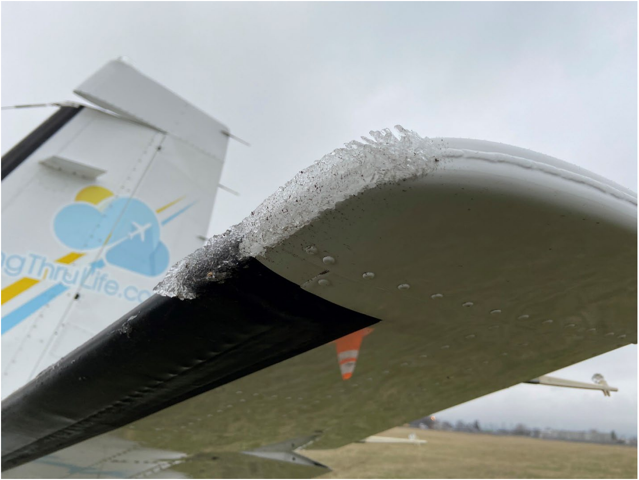
Figure 3: View of ice on leading edge of horizontal stabilizer. (Courtesy of FAA)
