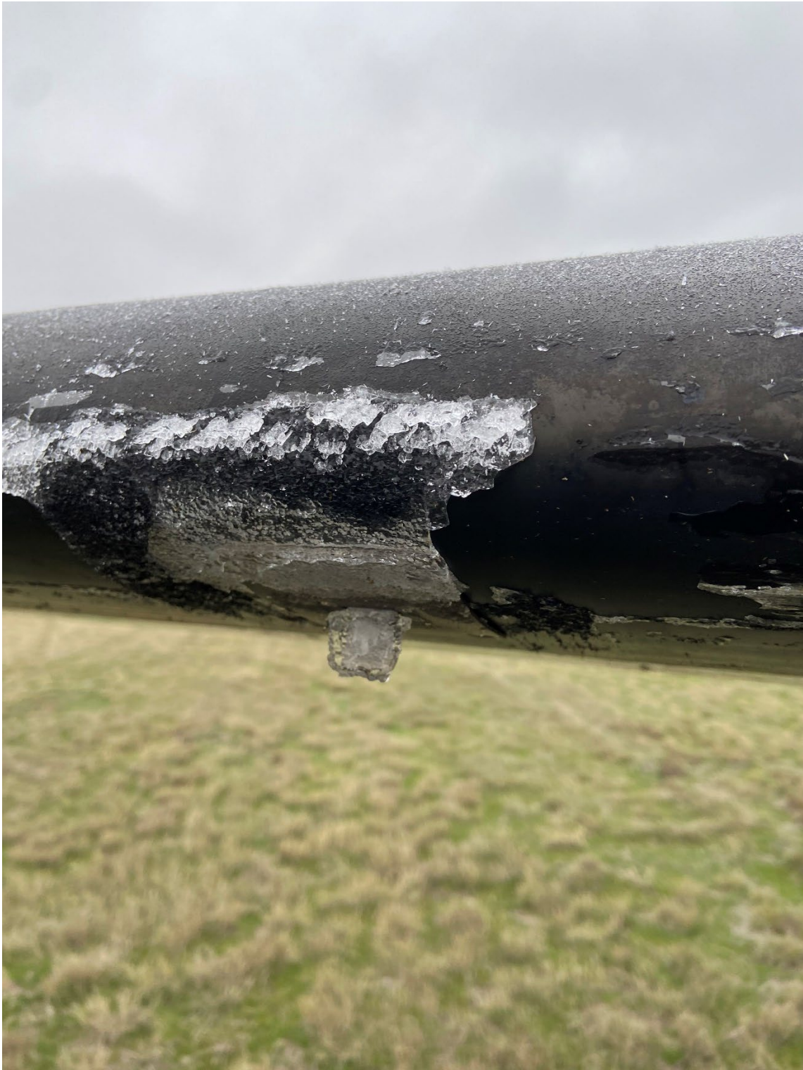
Figure 2: View of ice on stall warning vane (Courtesy of FAA)
